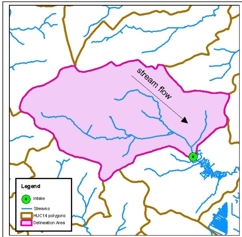
Figure 5. Example of a delineated source water assessment area to a water-supply intake
