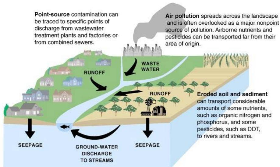
Figure 4. Schematic diagram of point and nonpoint sources of contamination showing how they can affect ground and surface-water quality.
