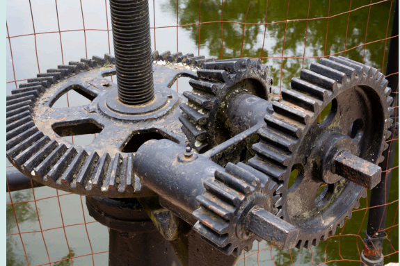
Delaware and Raritan Canal lock control gears in Bulls Island State Park.
