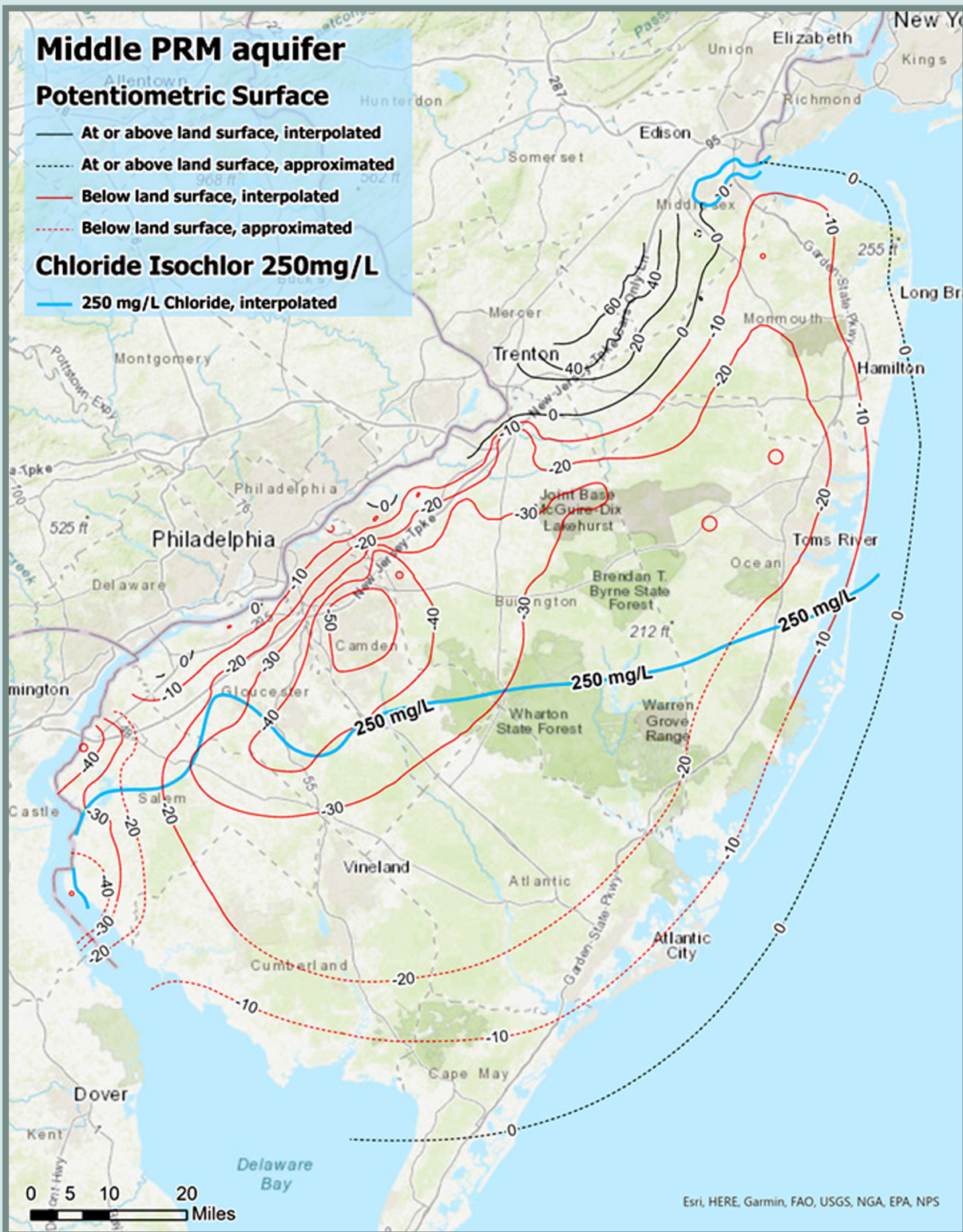
Figure C7. 250 mg/L isochlor line and potentiometric surface for Middle PRM Aquifer from the USGS report on the condition of New Jersey's confined aquifers in 2013, the most recent year for which such data is published.
