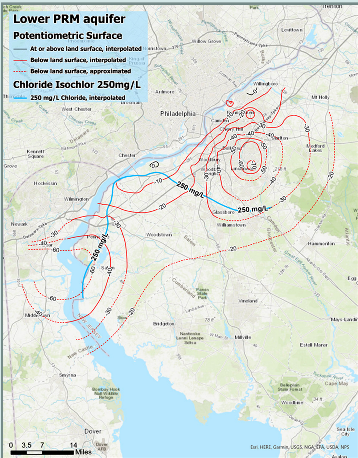
Figure C11. 250 mg/L isochlor line and potentiometric surface for Lower PRM Aquifer from the USGS report on the condition of New Jersey's confined aquifers in 2013, the most recent year for which such data is published.
