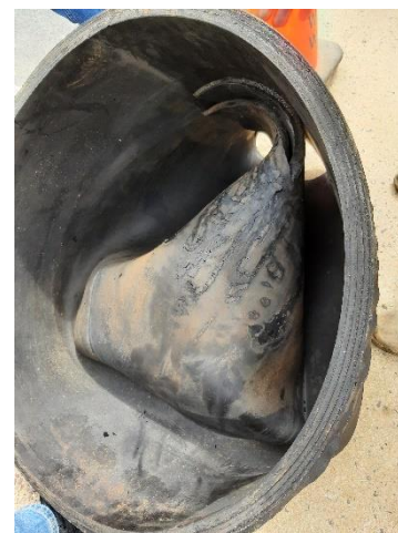
FIGURE 3: FAILED DUCKBILL CHECK VALVE
