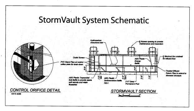
All maintenance plans incorporating the StormVault system must indicate that sediment be removed at or before the average depth of sediment reaches six (6) inches.
