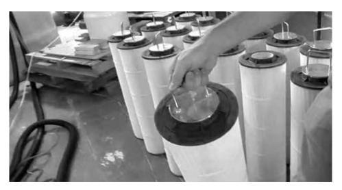
5. Once cleaned, install back into the vault. This completes maintenance. Ensure access lids are properly replaced.
