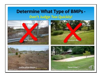
When performing maintenance work, it is important to know the type of BMP present and its design details, such as the minimum depth of sand, water depth, etc. Misjudgment of a BMP's type will not only result in ineffective maintenance, but also cause the BMP to fail. Therefore, it is important to know what type of BMP is present before performing the inspection and maintenance work.
