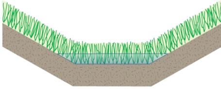
A grass swale is a stable, parabolic or trapezoidal channel that is lined with turf; it is used to improve water quality and convey stormwater runoff. Grass swales do not rely on the permeability of the underlying soil for pollutant removal; instead, pollutants are removed by settling and filtration through the grass. The maximum total suspended solids (TSS) removal rate is 50%.
