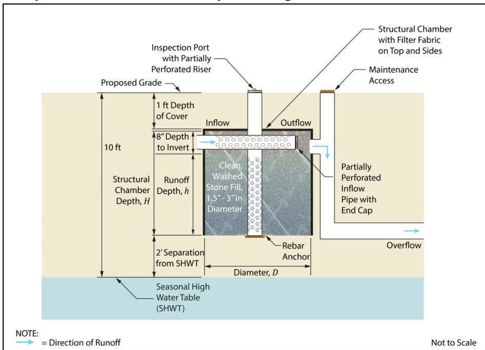
In this example, the depth to the seasonal high water table is 10 feet. Assuming 1-foot depth of cover, the allowable structural chamber depth,  $H$ , is calculated as follows, excluding any thickness of the top of the structural chamber and the required filter fabric:
