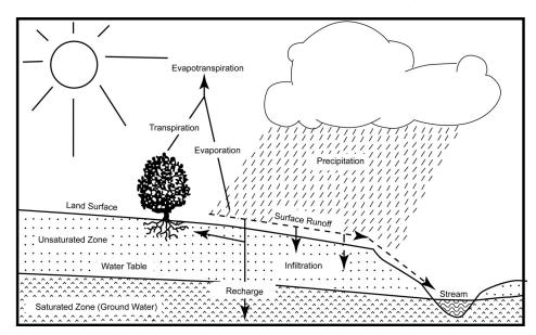
Figure 6-1: Groundwater Recharge in the Hydrologic Cycle
