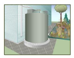
Cisterns are stormwater facilities that temporarily store stormwater runoff from rooftops, which is subsequently reused for non-potable uses, such as toilet flushing and vehicle washing. Cisterns can either be indoors or outdoors and above, at, or below grade. The reuse of the stormwater reduces the volume of stormwater runoff that makes it to downstream facilities. Take note that cisterns are not a viable stormwater management choice for sites with little or no demand for reuse.
