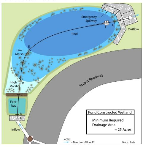
The table below shows the design criteria specific to pond constructed wetlands; for additional design criteria, refer to the *Basic Requirements* section of this chapter, beginning on page 3.
