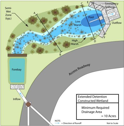
The illustration above shows the various components comprising a standard constructed wetland system from the extended detention category, for which a profile view taken along the centerline would look almost the same as a marsh constructed wetlands. Following the direction that stormwater runoff would take through the BMP; runoff enters the forebay and then flows over the spillway into the low and high marsh zones.
