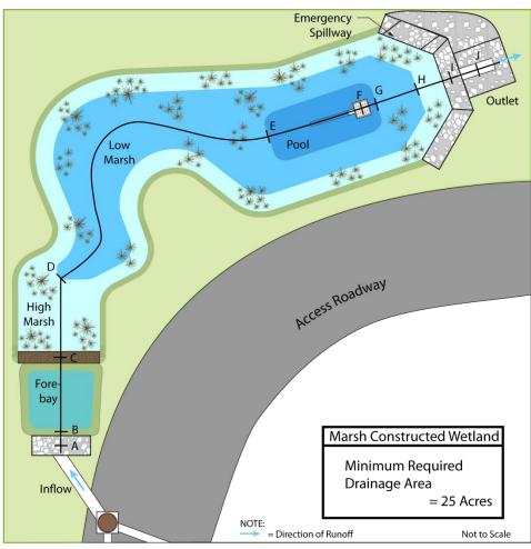
The table below shows the design criteria specific to marsh constructed wetlands; for additional design criteria, refer to the *Basic Requirements* section of this chapter, beginning on page 3.
