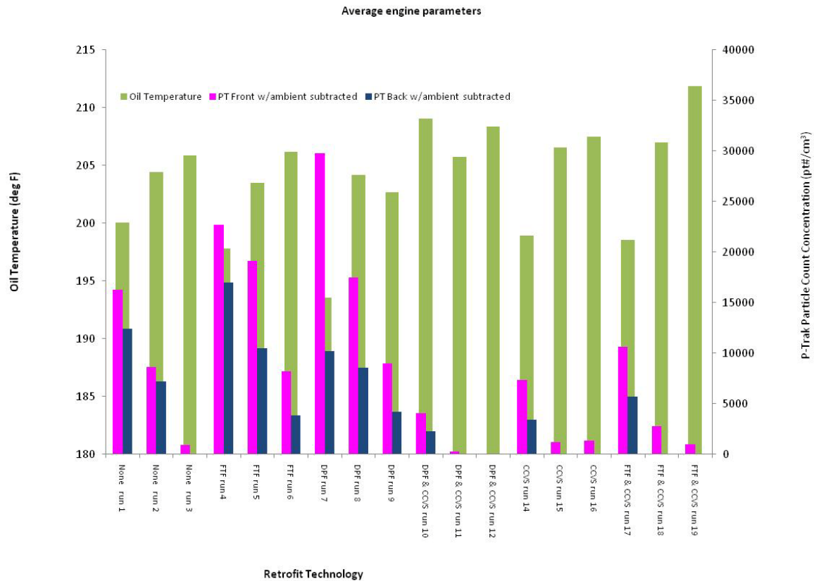
Figure 46: Trend between particle count results and engine oil temperature.
