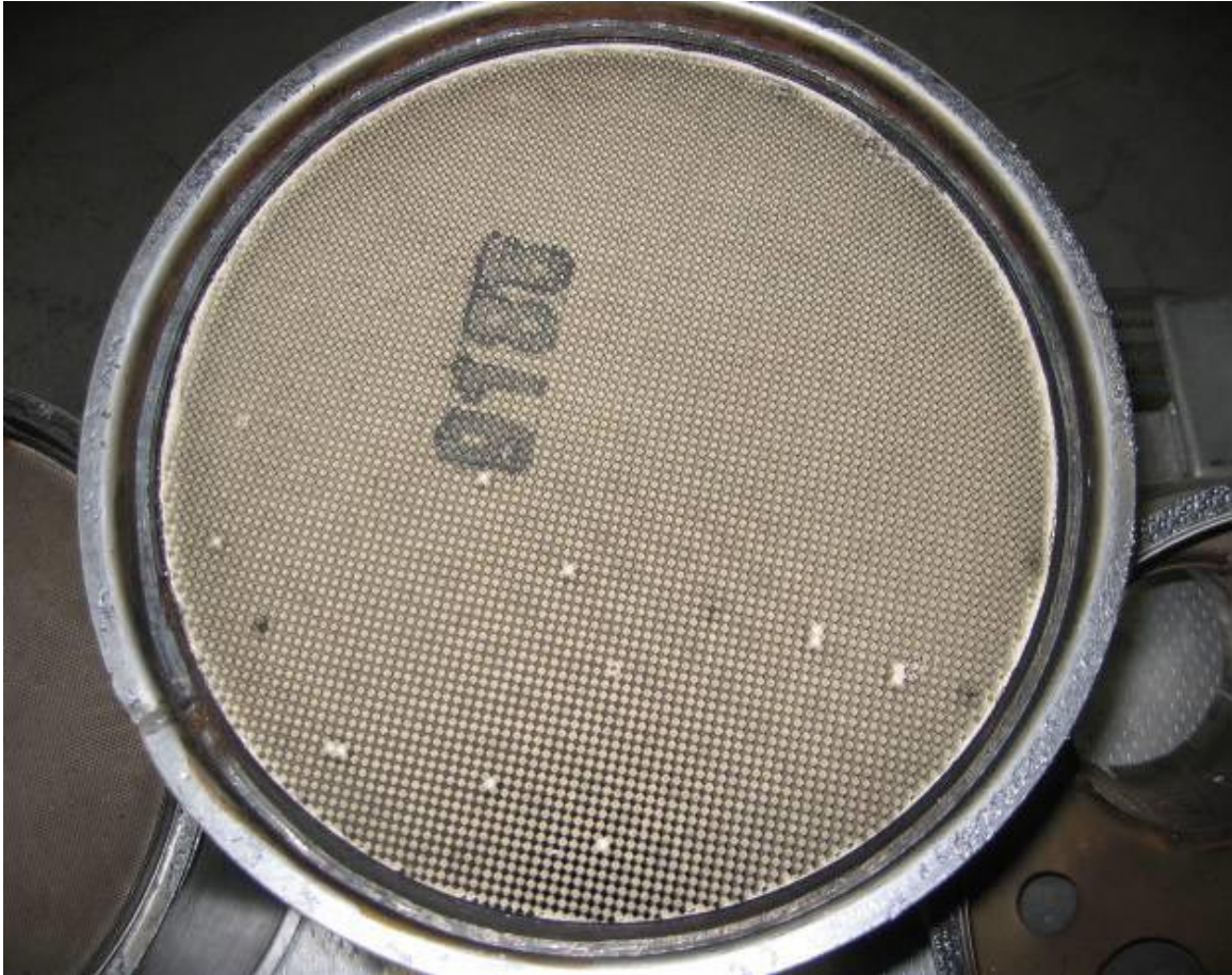
Figure 6: Exhaust intake face of DPF filter section during inspection.
