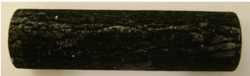
Figure 33: SEMTECH-D filter after three runs with the FTF and CCVS configuration.
