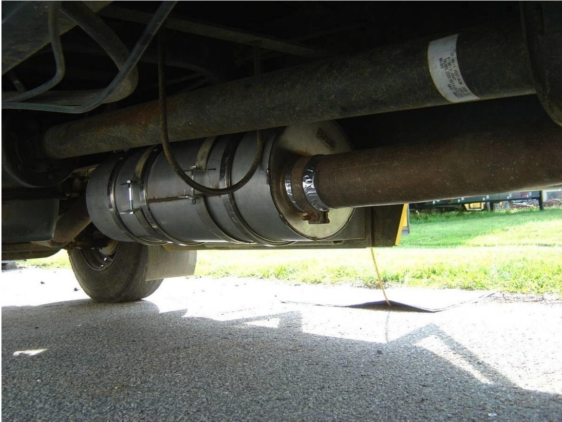
Figure 11: Johnson Matthey CRT, DPF, installed on the school bus.
