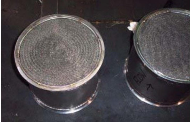
Figure 8: Internal component of the ESW Particulate Reactor ® . Source: M.J. Bradley & Associates, Inc. (2006) 11 .
