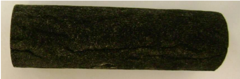
Figure 31: SEMTECH-D filter after use with three runs with no tailpipe retrofit for baseline condition.
