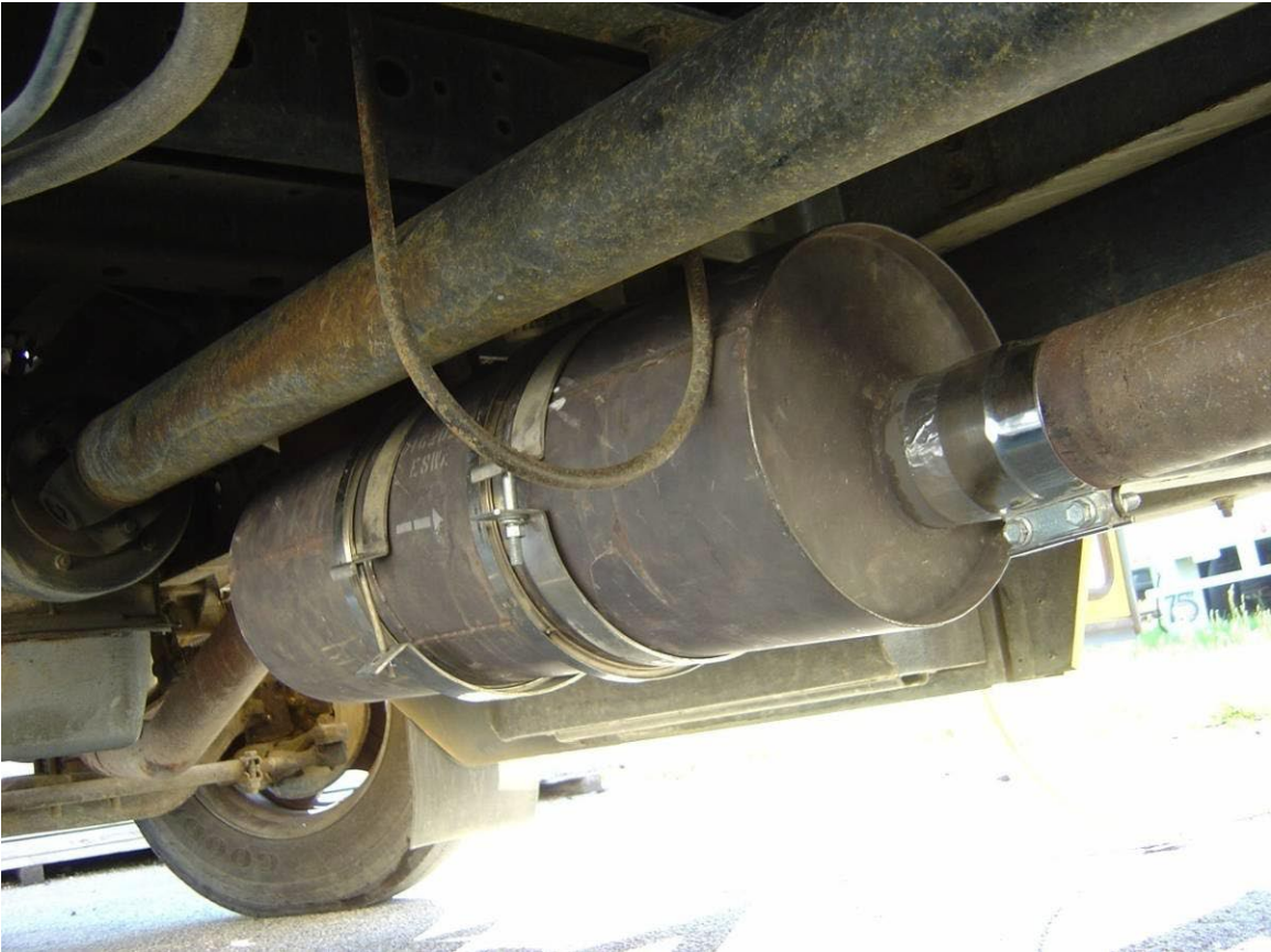
Figure 9: ESW Particulate Reactor (FTF) installed on the school bus.
