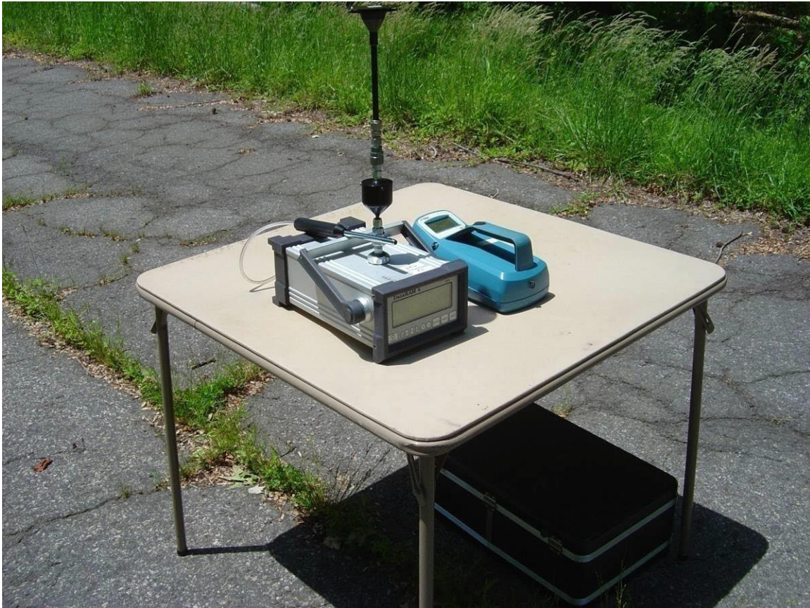
Figure 3: DataRAM and P-Trak instruments at ambient monitor station located 300 m from south west 0.1 mile turnaround loop.
