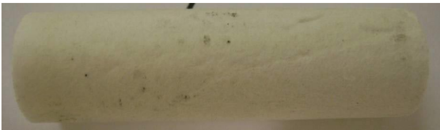
Figure 32: SEMTECH-D filter after use with three runs using the DPF & CCVS retrofits configuration.
