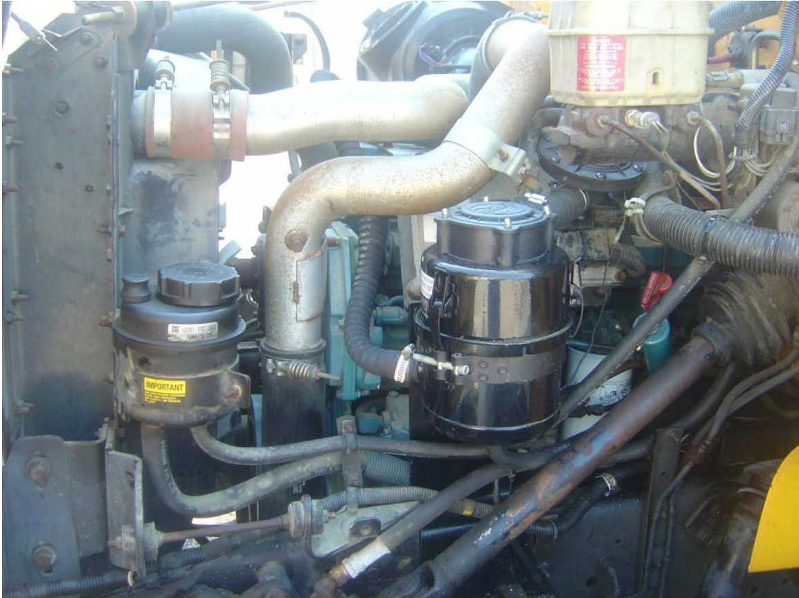
Figure 13: Donaldson Spiracle Crankcase ventilation system, CCVS, installed in the school bus tested.
