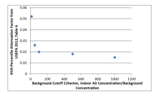
If instead the 95<sup>th</sup> upper confidence limit attenuation factors from Table 6 are plotted, all values are between 0.01 and 0.02 except for the cutoff criterion of ten times the background (see figure below).
