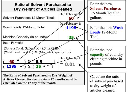
Note: All dry cleaning machines using a petroleum solvent, or the Non-HAP General Permit (GP-013) must calculate the ratio of solvent purchased to dry weight of articles cleaned. Check your compliance plan for this requirement.
