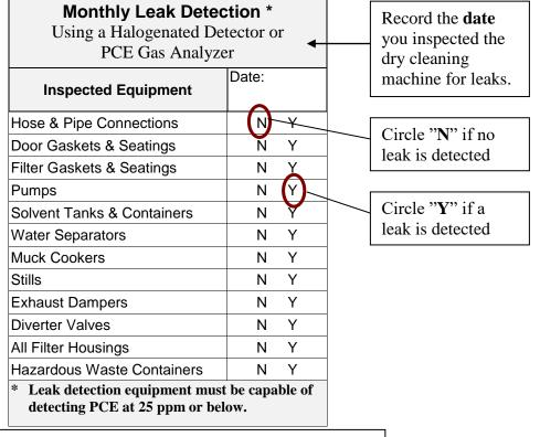
Note: If perchloroethylene is detected above regulated thresholds from the dry cleaning machine, the dry cleaning machine must be shut down until repaired.
