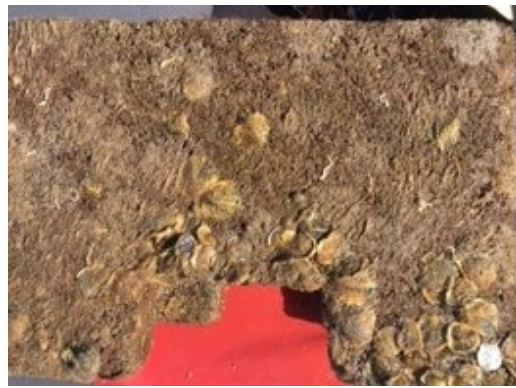
Fig. 13. Oyster spat set on concrete Reef Ball (left panel); oyster spat set on concrete Oyster Castle® and marine fouling organisms (middle panel); Oyster Castles® can be connected to create multiple widths and heights depending on site needs (right panel). Images courtesy of Dr. B. Ravit.
