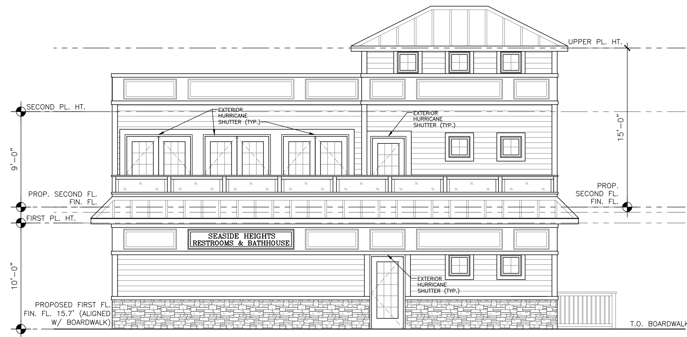
1 FRONT ELEVATION @ BOARDWALK SCALE: \frac{3}{16} " = 1'-0"
