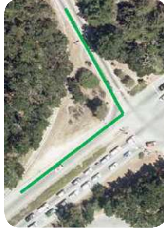
This high-speed ramp has been replaced with a 90-degree intersection. Image: California Department of Transportation
