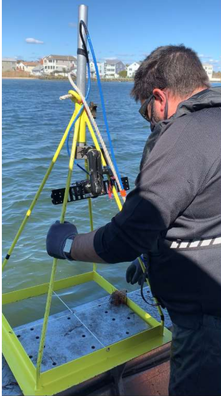
Figure 3. Quadrat Frame with Mounted GoProHero3 for SAV Sampling.
