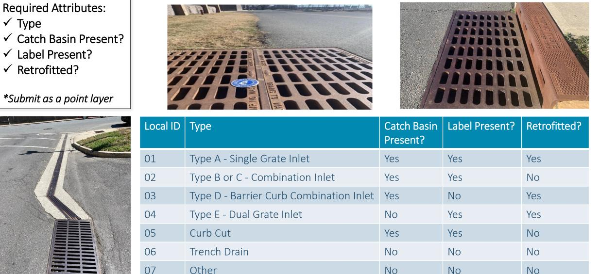
"Catch Basin" means a cistern, vault, chamber, or well that is typically built along a street and below an inlet grate as part of the storm sewer system that is designed to capture and retain sediment, debris, and pollutants so those particles do not pass on to the stormwater sewer system.
