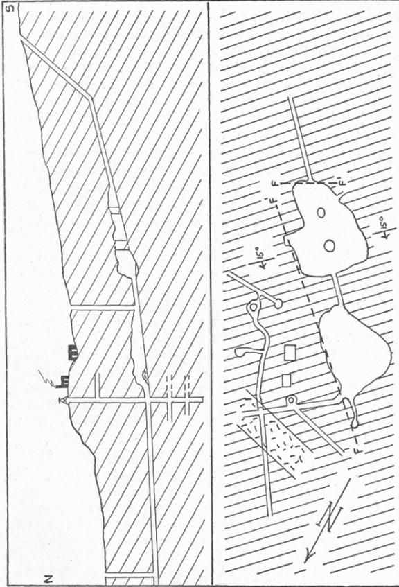
FIG. 9. Section at the Griggstown copper mine. The upper figure shows the extent of the workings, the lower figure a plan of the chambers at the 100-foot level. A dike of diabase is reported along the drain tunnel north of the main shaft. (After J. D. Gabel.)
