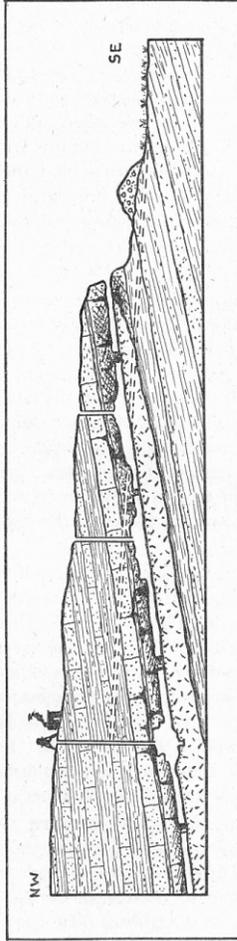
FIG. 4. Generalized cross-section through the old Schuyler copper mine at Arlington, New Jersey. The mine workings followed the upper surface of the thin Arlington sill, here about 20 feet thick. Mineralized zones follow the top contact of the sill in beds of sandstone. The numerous shafts are now concealed, and the locality is a residential suburb. The position of the main drain is indicated by dotted lines.
