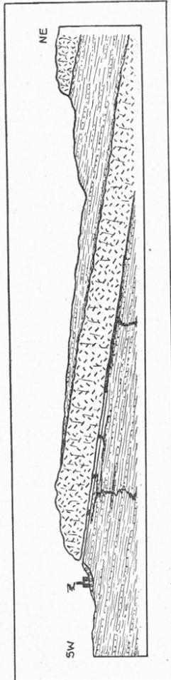
FIG. 7. Generalized cross-section at the American copper mine near Somerville, New Jersey. The main workings followed the under surface of the basaltic flow of First Watching Mountain.
