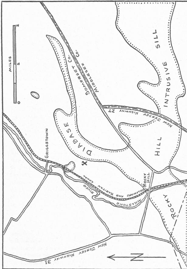
FIG. 8. Generalized sketch map of the Griggstown area showing location of the old Griggstown copper mine and the outcrop of the nearby Rocky Hill intrusive diabase sill.
