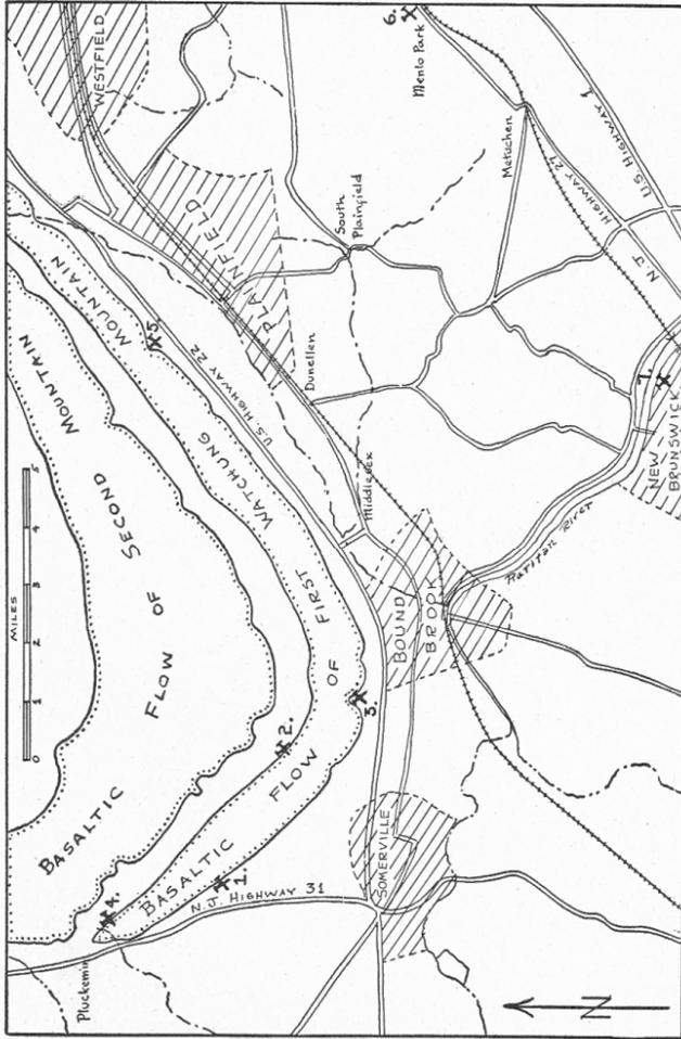
FIG. 6. Generalized sketch map of the Somerville-New Brunswick area, New Jersey, showing the location of several old copper mines and the surface outcrops of the basaltic flows of the Watchung Mountains. Numbered copper prospects or mines are as follows: 1. American or Bridgewater mine; 2. Bolmer prospect; 3. Chimney Rock mines; 4. Hoffman prospect; 5. Green Valley prospects; 6. Menlo Park mine; 7. New Brunswick (French) mine.
