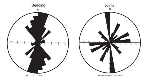
Figure 3. Structural data on rocks in study area. Joints not present in all exposures.
