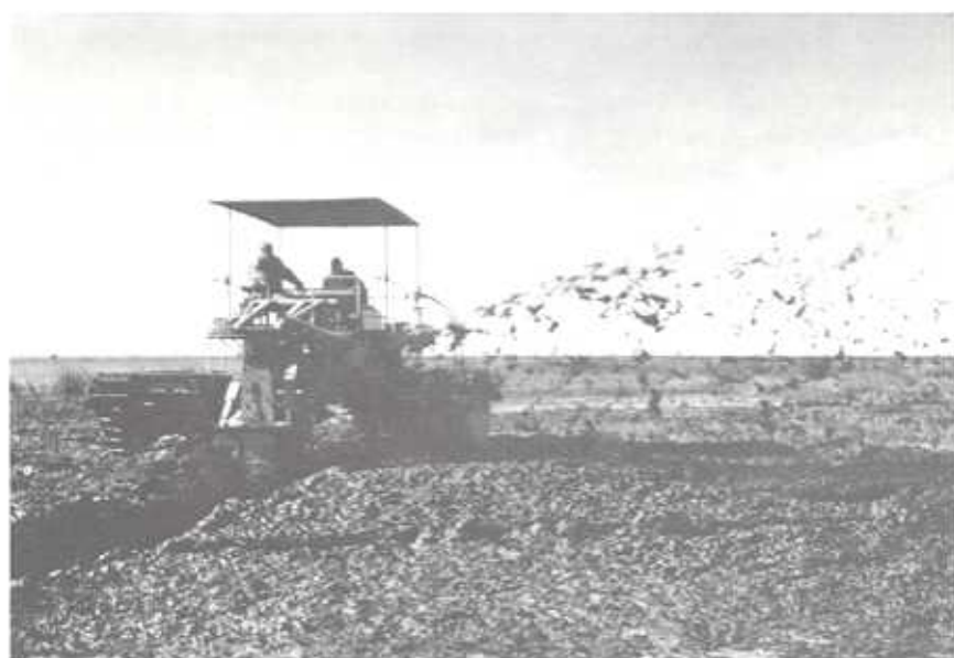
Fig. 2 Most of the problems associated with improper sod disposal have been eliminated by this new amphibious rotary ditcher.
