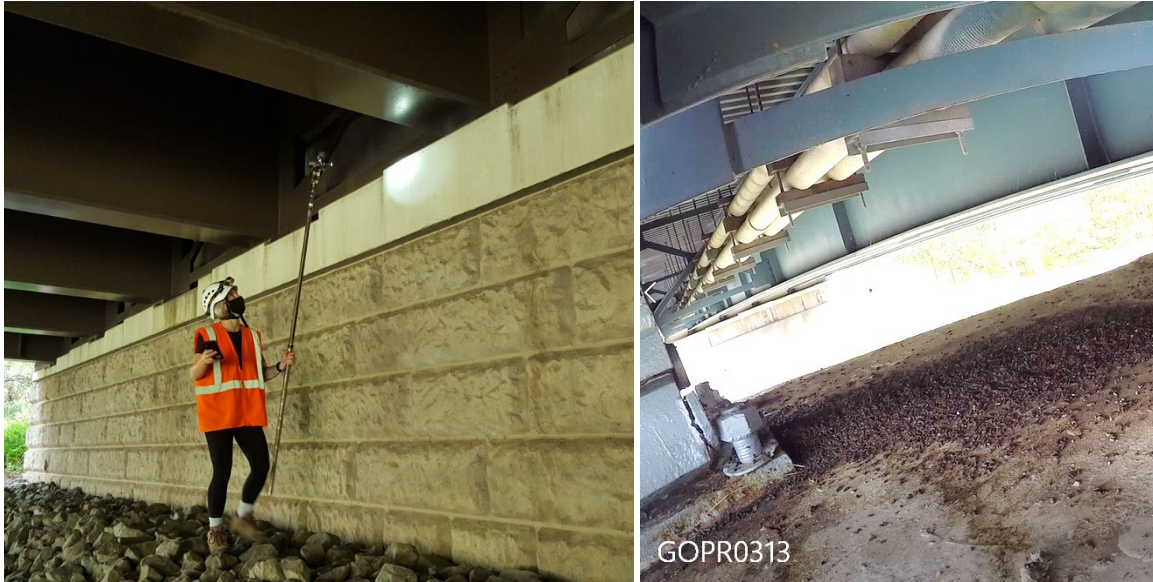
Figure 1. Personnel using a telescoping video camera array to inspect bridge abutment ledges (at left) and pier caps (at right) during bridge bat surveys. A large pile of bat guano confirms the presence of bats in the photo at right.
