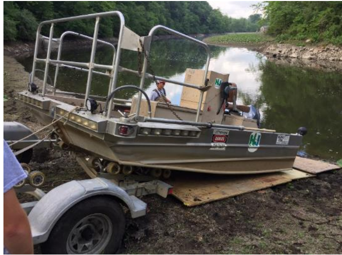
NJDFW staff using plywood to launch an electrofishing boat in partially lowered Columbia Lake
