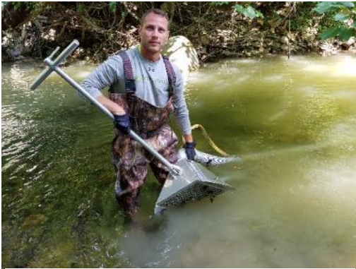
Equipment used to vacuum sediment from the streambed.
