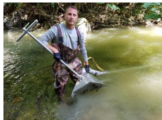
Equipment used to vacuum sediment from streambed.
