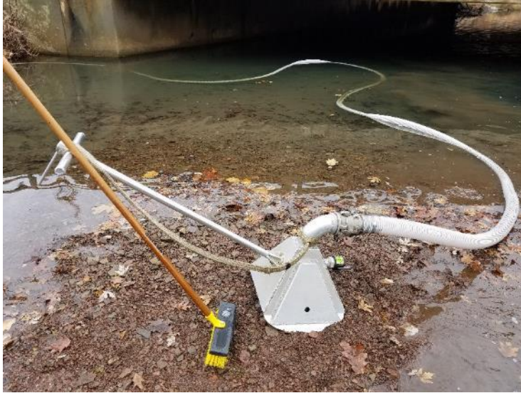
Equipment used to vacuum sludge from the streambed of the First Neshanic River.
