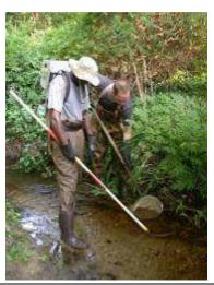
by battery or generator, has been used almost exclusively since 1980. A battery-powered D.C. backpack unit, having one paddle-type electrode and used by an operator and one or two netters, has been in used since 1980 to sample small streams. On larger streams a gas generator is used in conjunction with a conversion box (to convert A.C. to D.C.), two or three electrodes, and a five to seven person field crew.
