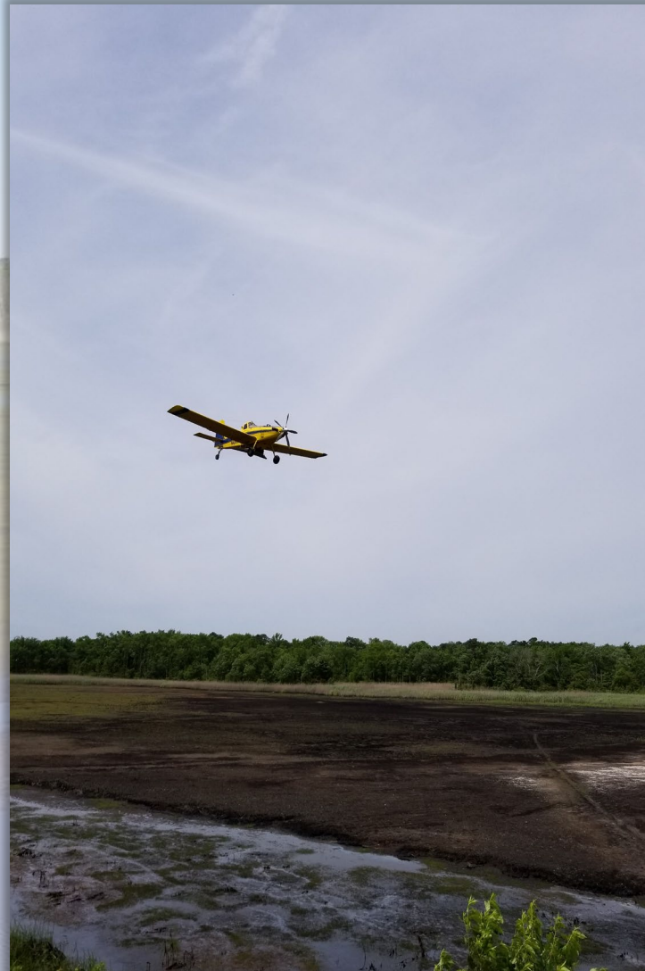
AgCat Aerial Seeder spreading wetland seed mixture over impoundment Mallard in June 2019
