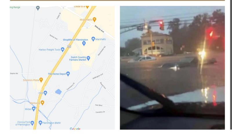
The extreme rainfall overwhelmed existing storm sewer systems resulting in flooding along roadways far from any streams
