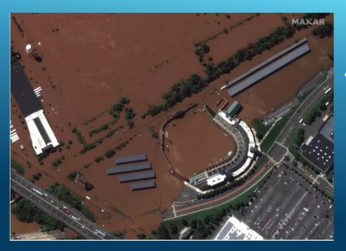
Flooding peaked roughly at FEMA's 500-year flood elevation (41.0 ft NAVD) which is 2.8 ft above FEMA's 100-year flood elevation (38.2 ft NAVD).
