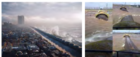
Figure 1a: Our visualisation of a pneumatic storm surge barrier positioned along the Rockaway Peninsula (NYC) and b the inflation of the Ramspol Balgstuw between two lakes (clockwise image credit martiennieuws.nl)
