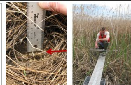
Left: Accretion being measured above feldspar horizon, Right: SET measurement being performed by field researcher Joe Grzyb. The plank is used to minimize disruption of the SET Plot area.
