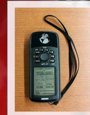
Figure 5: The GPS 72 used to obtain the coordinate locations of the fire hydrants.
