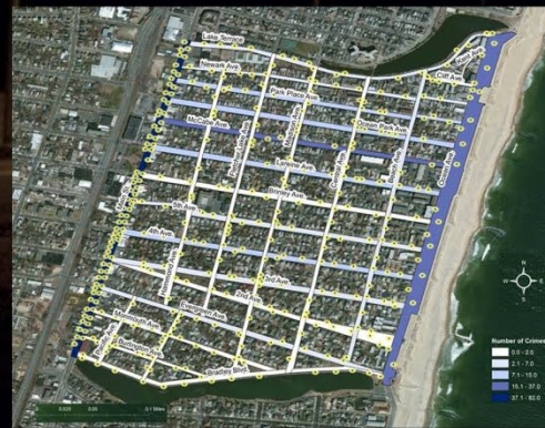
Figure 3: Aerial footage of Bradley Beach, NJ. Bottom layer displays each street color coded based upon the number of crimes committed there. Top layer displays each streetlight in Bradley Beach, along with the approximated area illuminated by each light.
