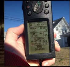
Figure 4: GPS unit used to collect coordinate locations of streetlights in Bradley Beach, NJ.
