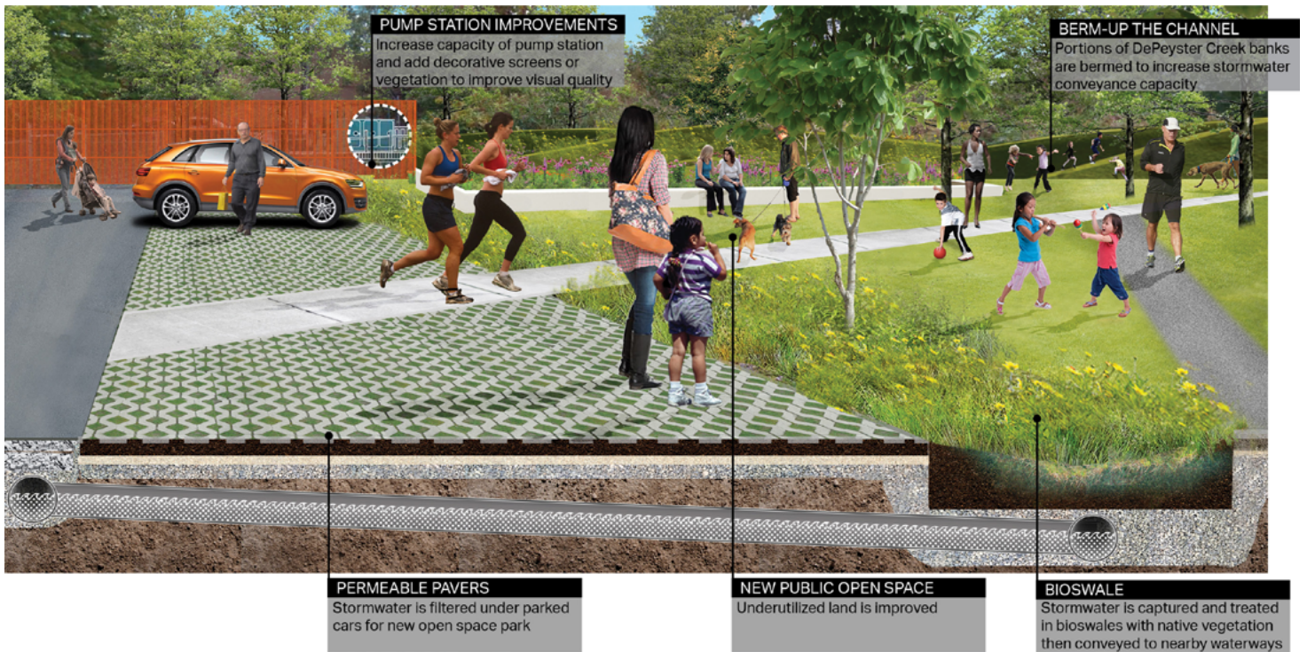
Example Rendering of a Potential Drainage Improvement Concept Near DePeyster Creek Pump Station
