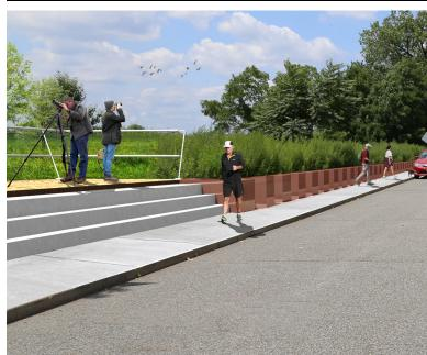
Alternative 1 would implement a line of protection around the Project Area that would quard against flooding from the Hackensack River and Berry's Creek during coastal storm surges. Alternative 1 would be designed to provide flood protection up to an elevation of 7 feet (NAVD 88). This height would provide protection against approximately the present-day 50-year storm surge. Public realm and ecological benefits would also be incorporated.
