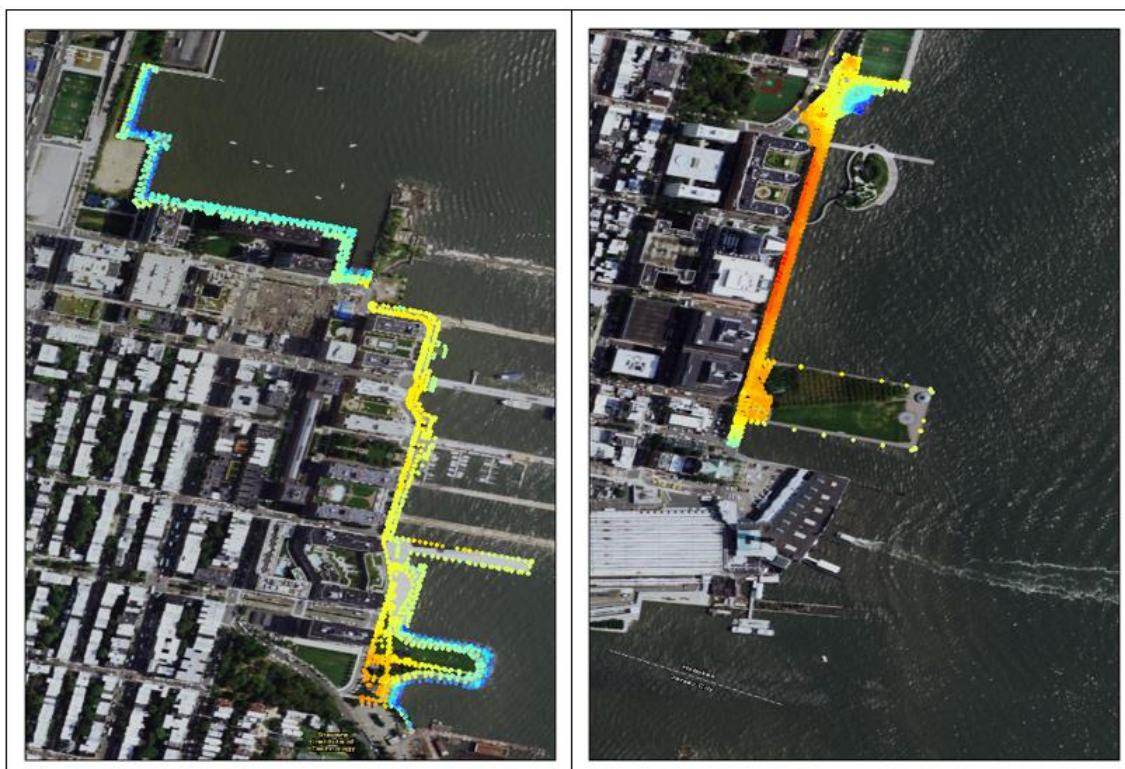
Figure 3-6. Topographic Survey Data Collected Along Portions of Hoboken Waterfront in July 2015 (Northern Portion in Left, and Southern in Right)
