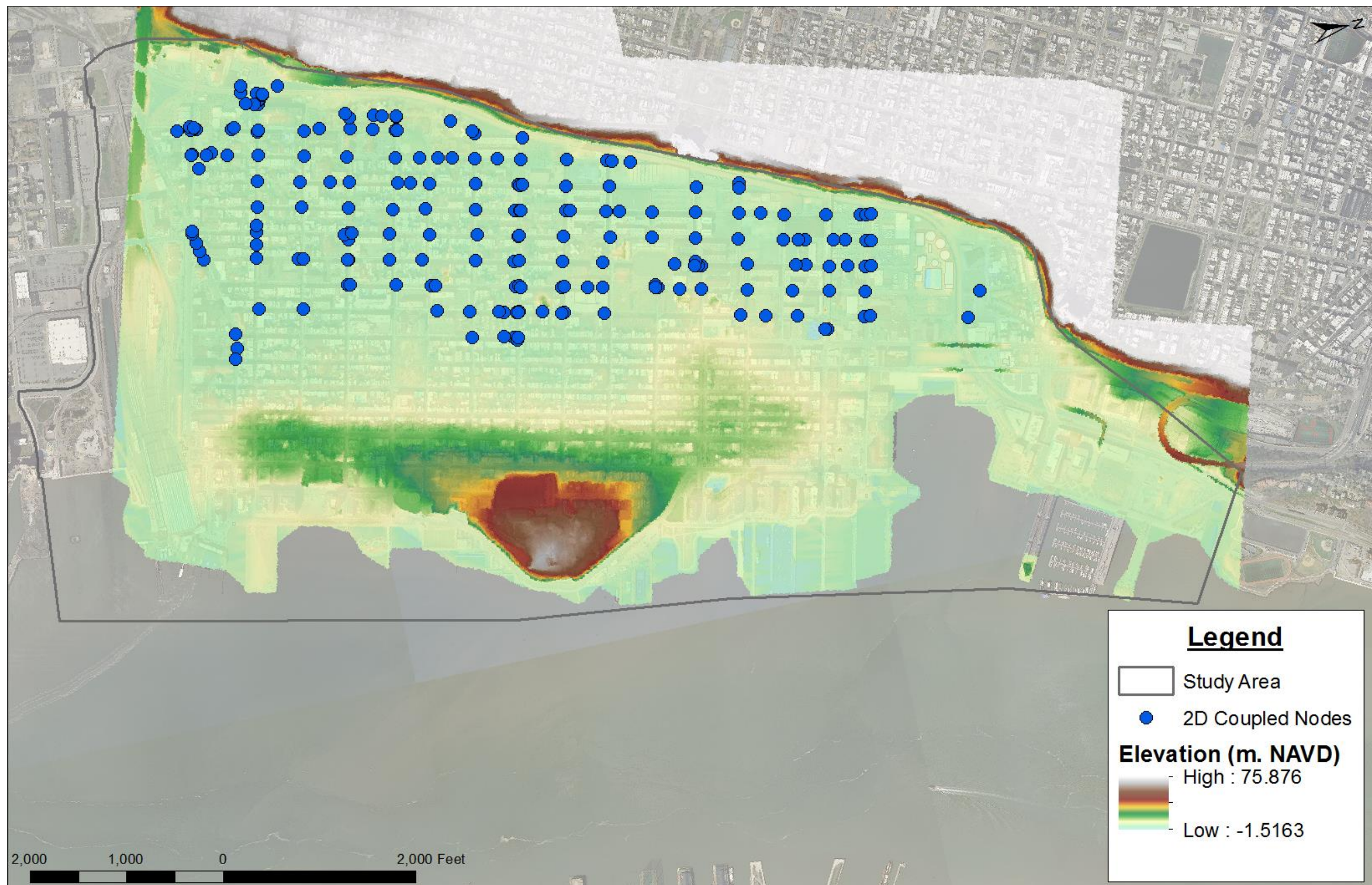
Figure 7-15. MIKE URBAN 2D Topography and Coupled Nodes
