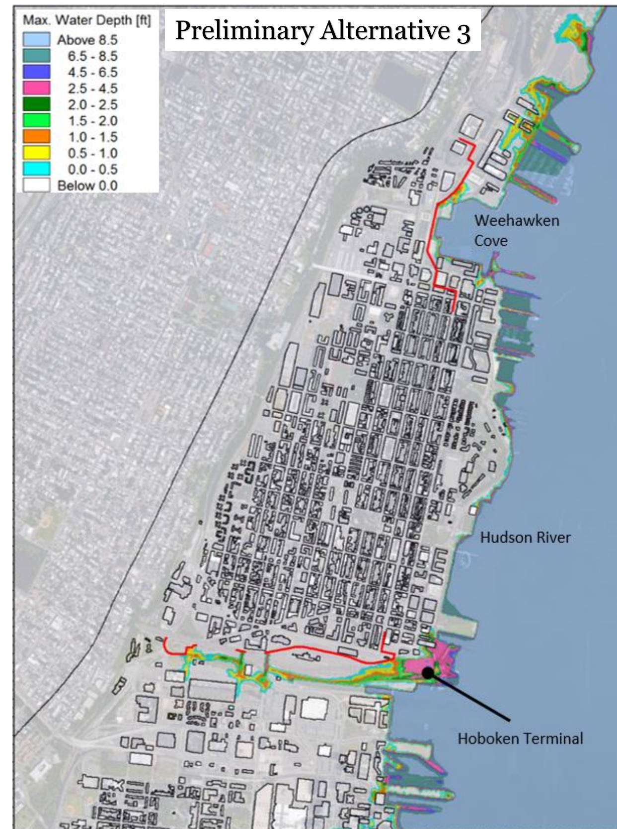
Figure 6-4. Comparison of the Flood Inundation and Maximum Water Depth in the Study Area during a 10% (10-year) Annual Chance Coastal Storm Surge Event
