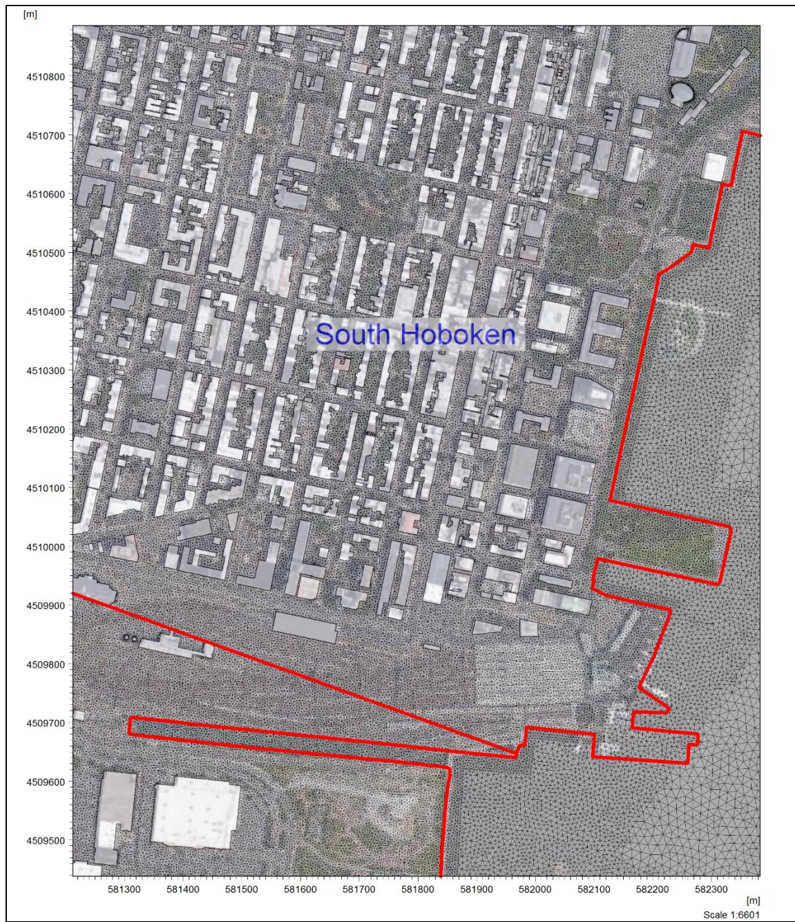
Figure 3-4. Mesh Resolution along the Southern Portion of Hoboken (red line is the municipal boundary)
