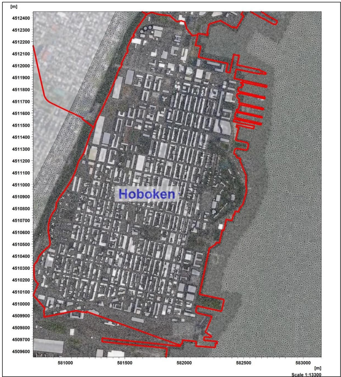
Figure 3-3. Mesh Resolution along the Streets of Hoboken and Adjacent Open Areas (red line is the municipal boundary)
