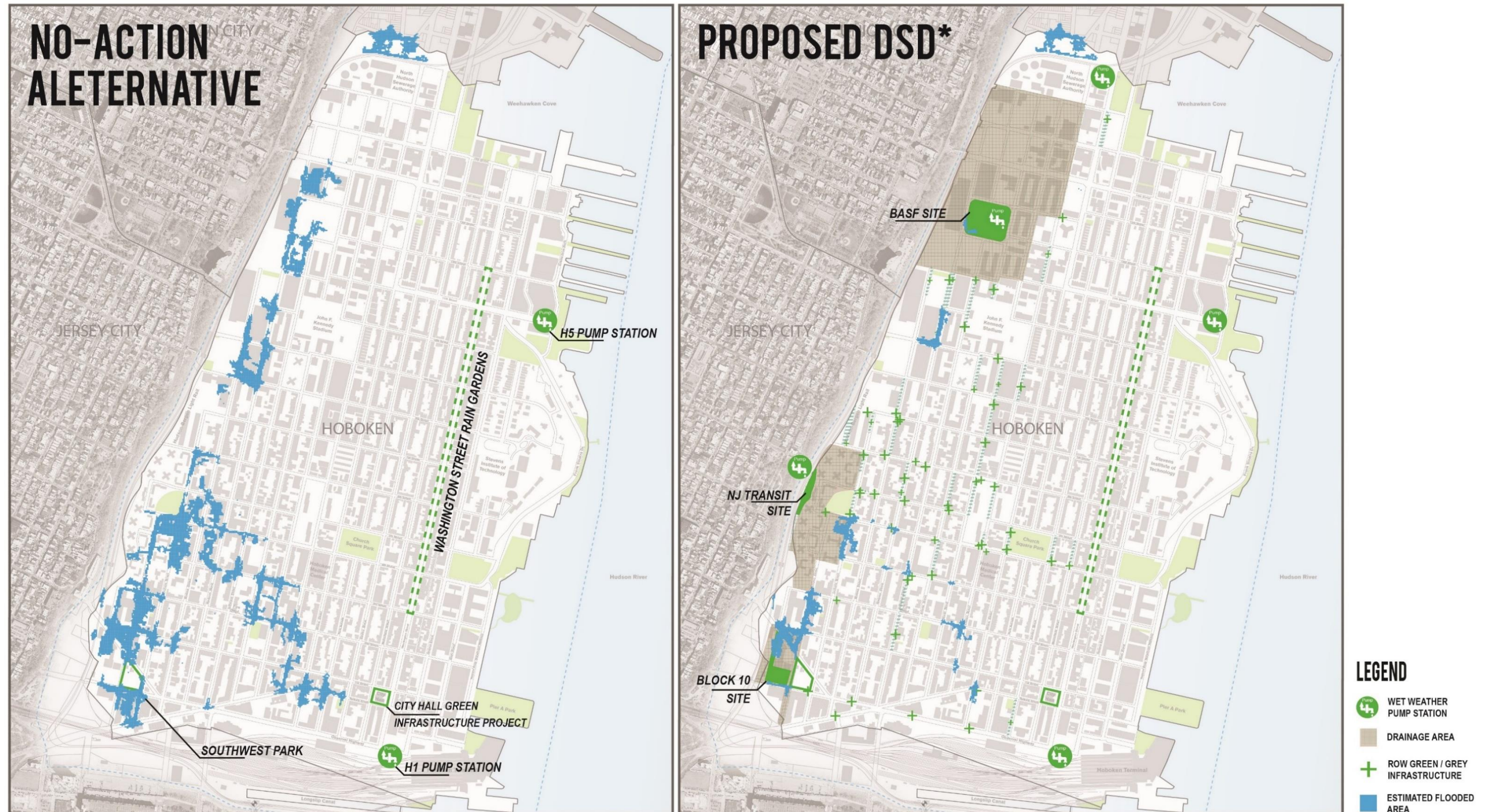
Figure 9-14. Comparison of NAA and Proposed DSD Alternatives 5-Year High Tide Results
