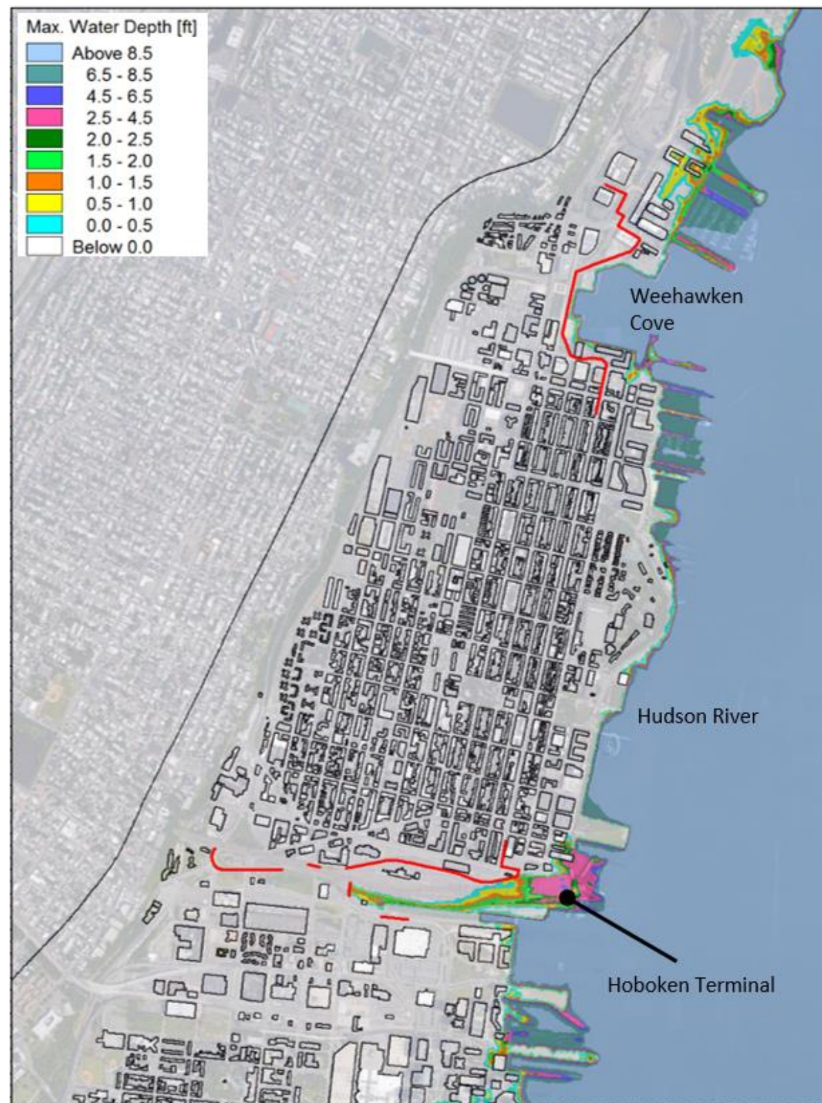
Figure 6-20. Spatial Plot Showing Maximum Flood Depths and Inundation Extents for the 2% Annual Chance Coastal Storm Surge Event (50-Year) with Alternative 2 (15 th Street)
