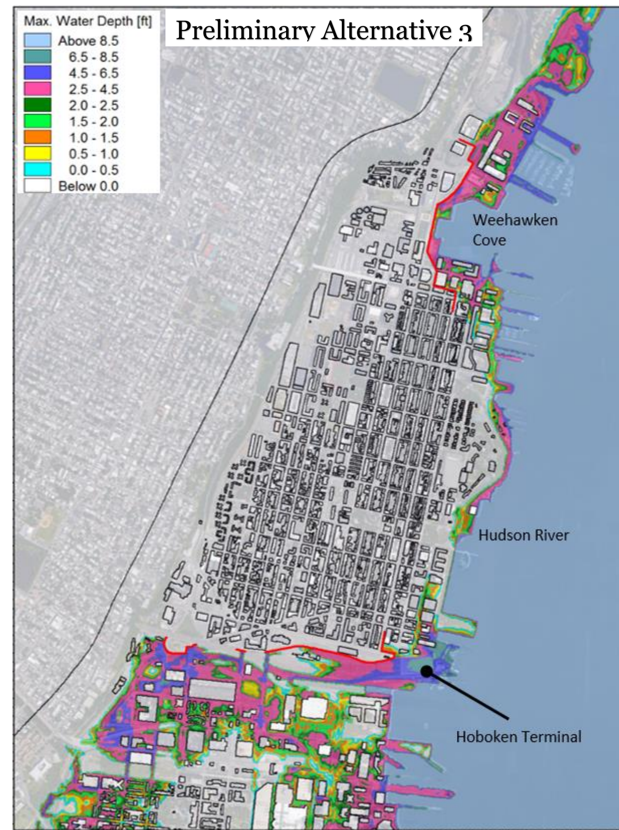
Figure 6-8. Comparison of the Flood Inundation and Maximum Water Depth in the Study Area during a 1% (100-year) Annual Chance Coastal Storm Surge Event
