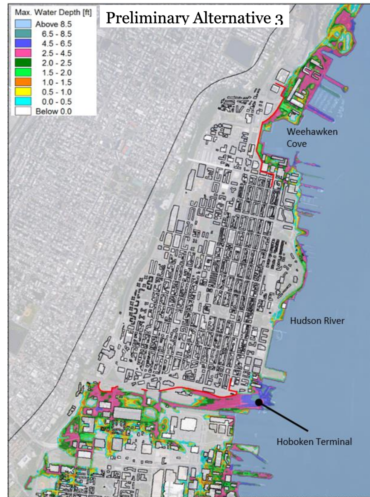
Figure 6-6. Comparison of the Flood Inundation and Maximum Water Depth in the Study Area during a 2% (50-year) Annual Chance Coastal Storm Surge Event
