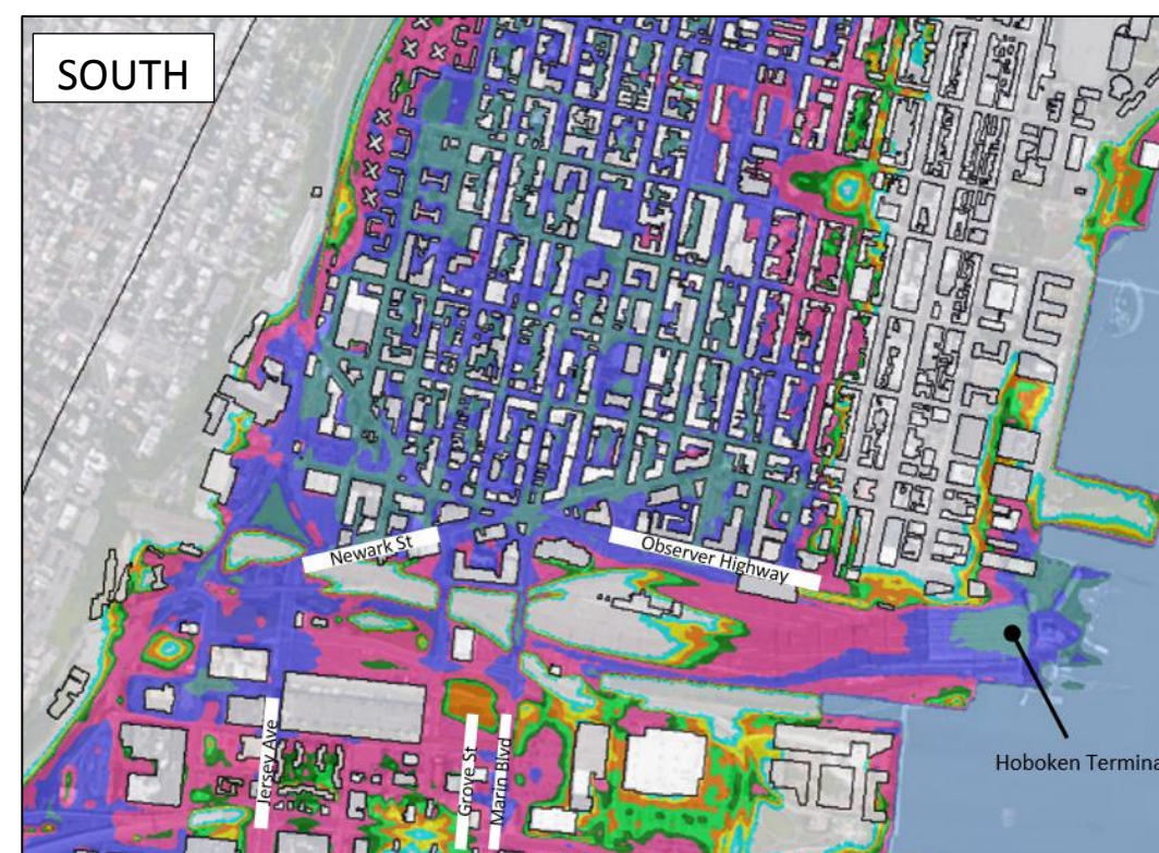
Figure 5-4. Flood Inundation and Maximum Water Depth in the Study Area during a 1% (100-year) Annual Chance Coastal Storm Surge Event
