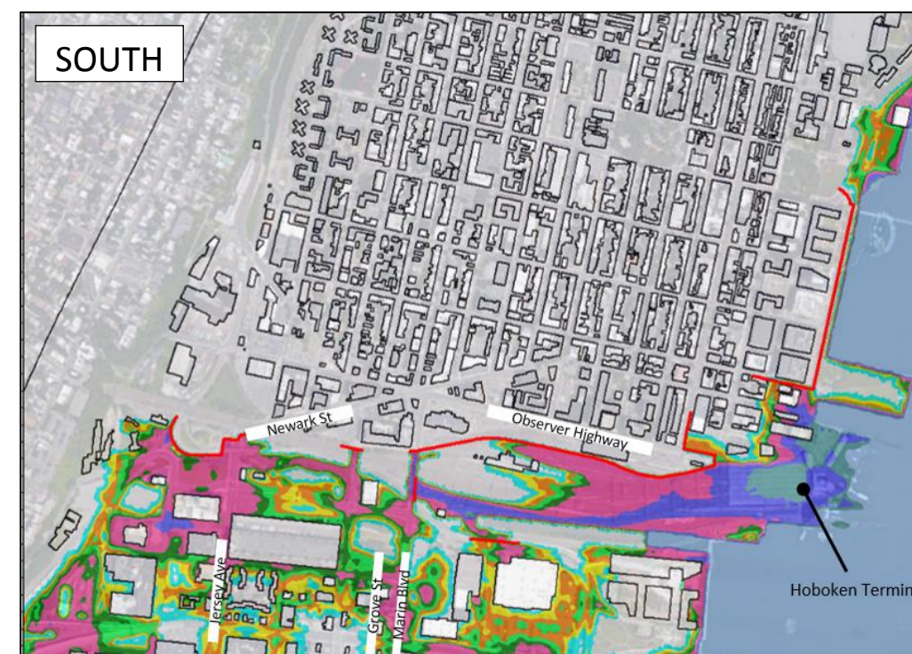
Figure 6-16. Spatial Plot Showing Maximum Flood Depths and Inundation Extents for the 1% Annual Chance Coastal Storm Surge Event (100-Year) with Alternative 1 (Waterfront)
