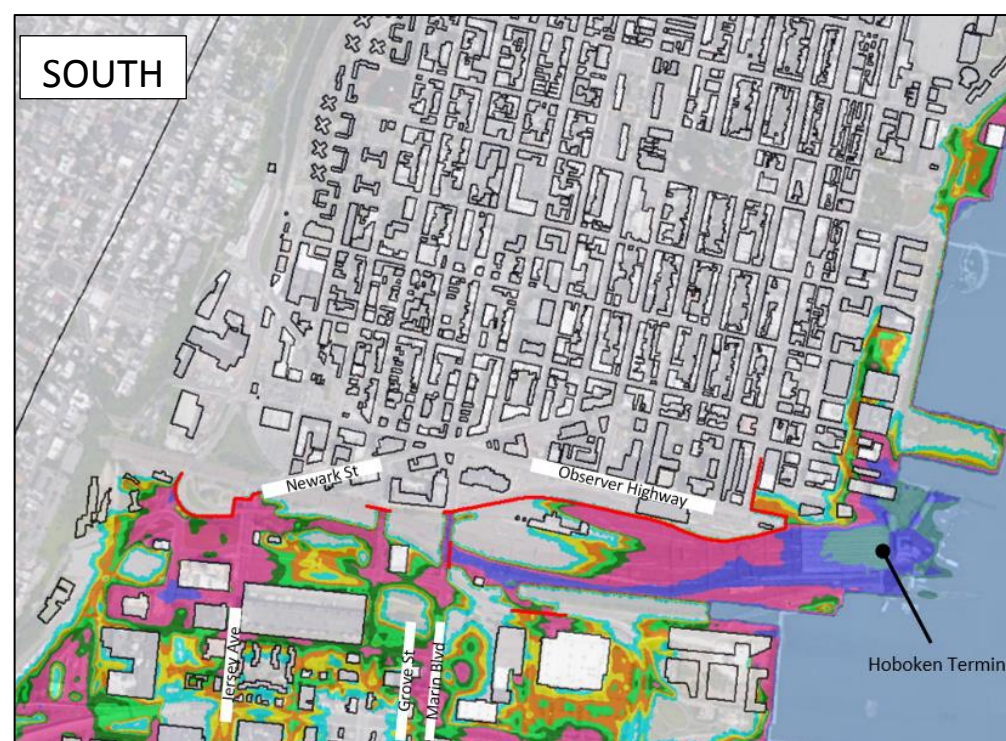
Figure 6-26. Spatial Plot Showing Maximum Flood Depths and Inundation Extents for the 2% Annual Chance Coastal Storm Surge Event (50-Year) with Alternative 3 (Alleyway)
