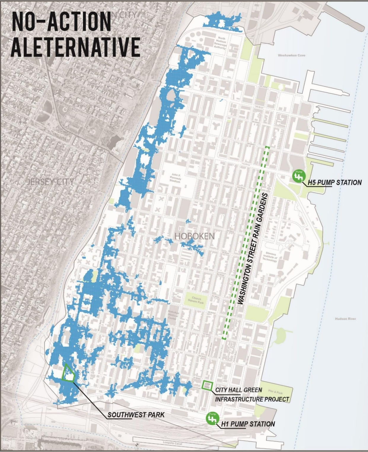
*DSD (DELAY/STORE/DISCHARGE) ARE COMPONENTS OF PROPOSED STORMWATER MANAGEMENT Figure 9-18. Comparison of NAA and Proposed DSD Alternatives 25-Year High Tide Results
