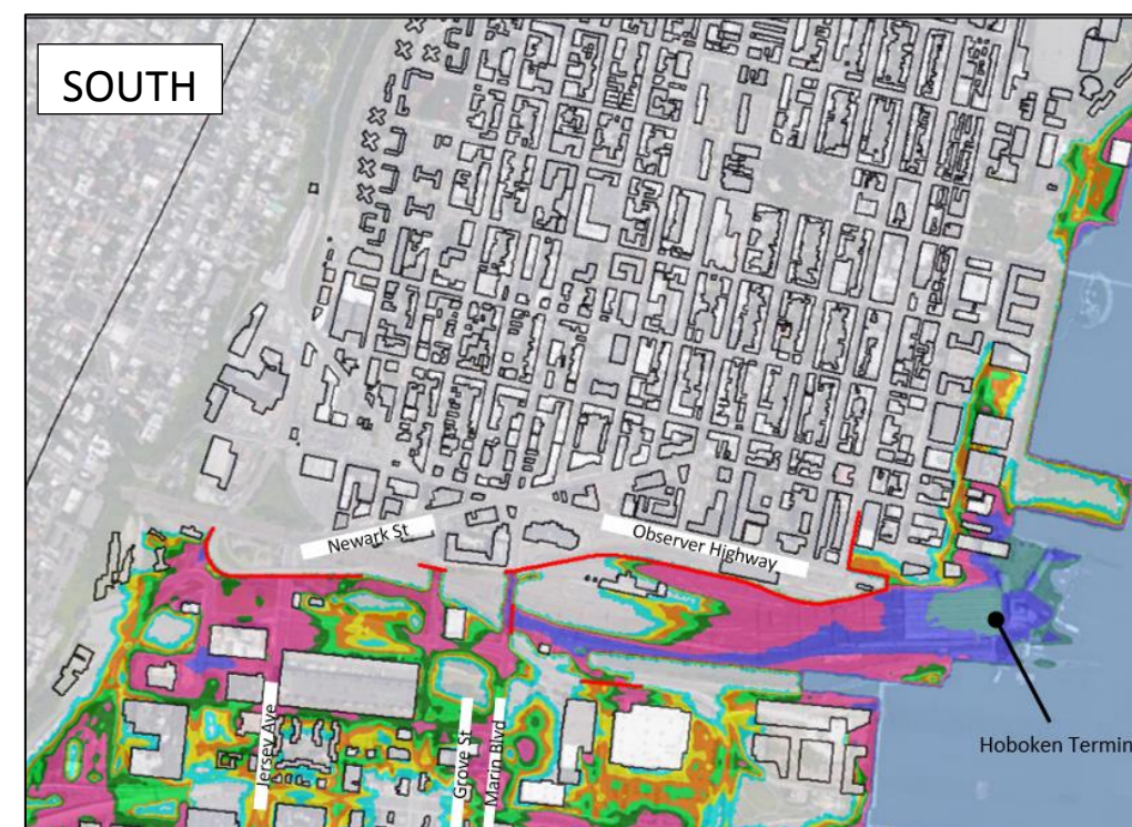
Figure 6-22. Spatial Plot Showing Maximum Flood Depths and Inundation Extents for the 1% Annual Chance Coastal Storm Surge Event (100-Year) with Alternative 2 (15 th Street)
