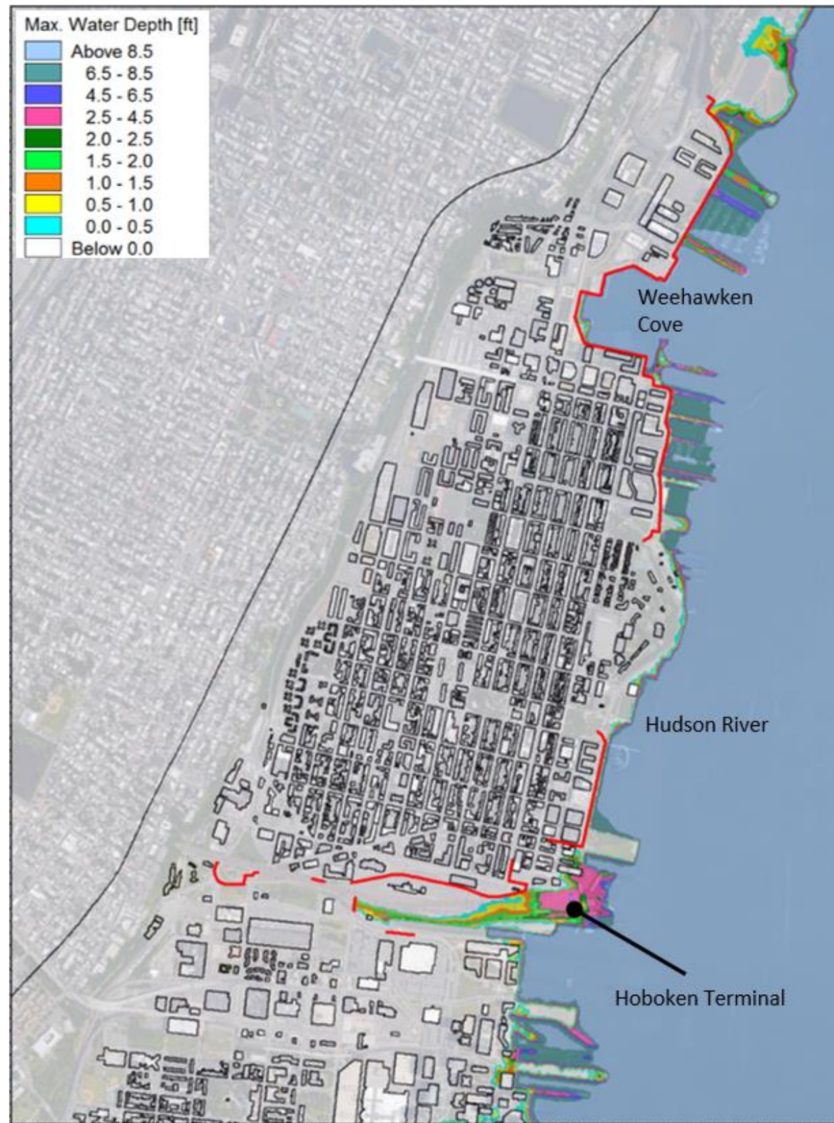
Figure 6-12. Spatial Plot Showing Maximum Flood Depths and Inundation Extents for the 10% Annual Chance Coastal Storm Surge Event (10-Year) with Alternative 1 (Waterfront)
