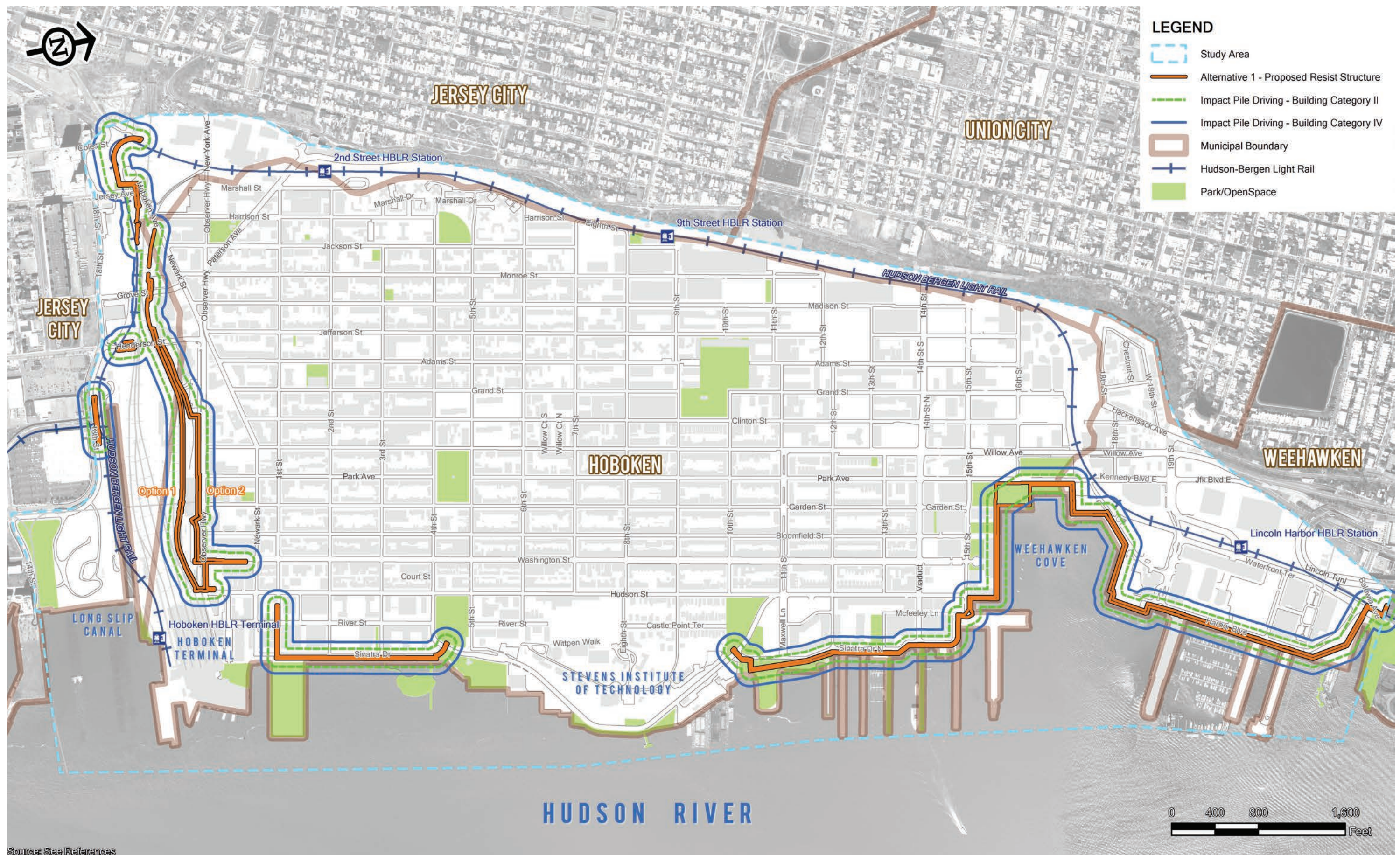
Figure 4.49 Structural Damage - Impact Pile Driving- Alternative 1
