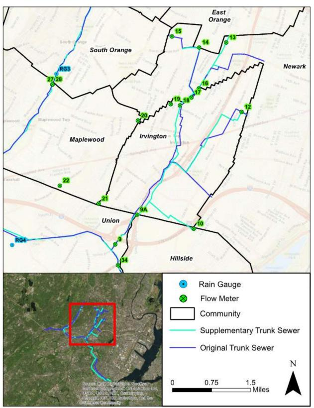
Figure 4-3 Flow Meter and Rain Gauge Locations – Northern Service Area
