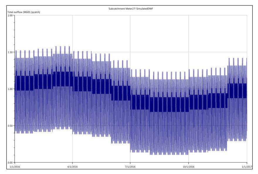
Figure 4-11 Simulated Dry Weather Flow for Subcatchment 27 during 2016 Model Simulation
