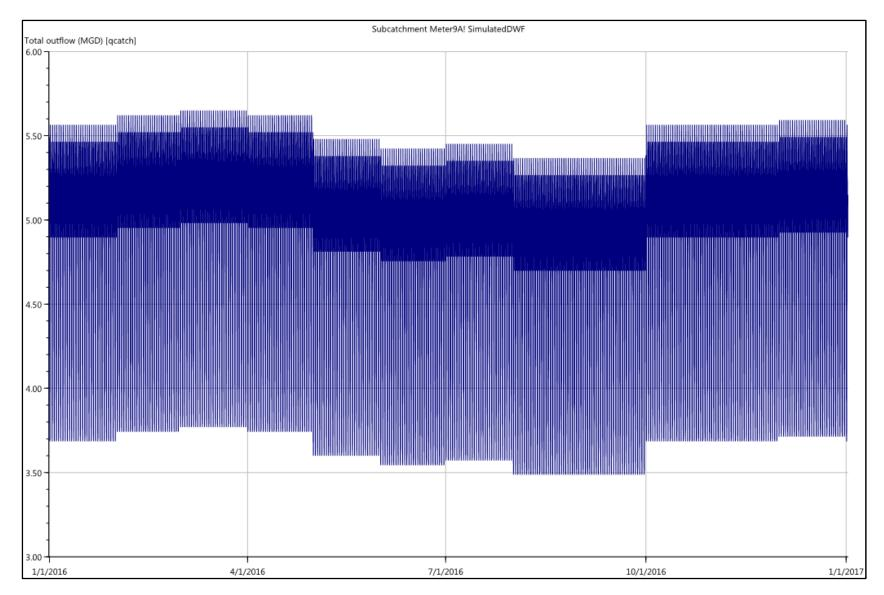
Figure 4-12 Simulated Dry Weather Flow for Subcatchment 9A during 2016 Model Simulation
