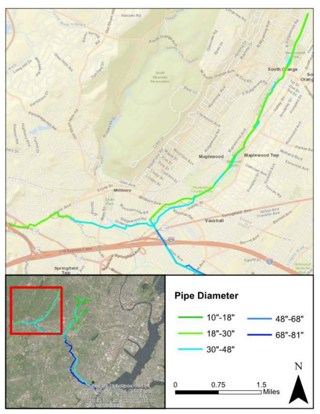
Figure 2-4 JMEUC Trunk Sewer Pipe Sizes and Shapes – Northwest Portion of Service Area
