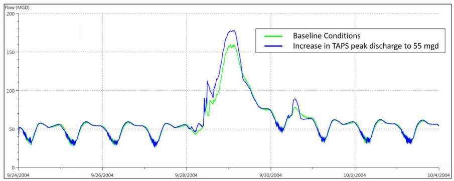
Figure 7-25 Simulated WWTF (Primary Effluent) Flow Rate with Increased TAPS Discharges
