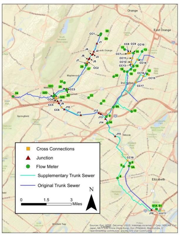
Figure 7-5 Locations of Modeled Junctions and Cross Connections
