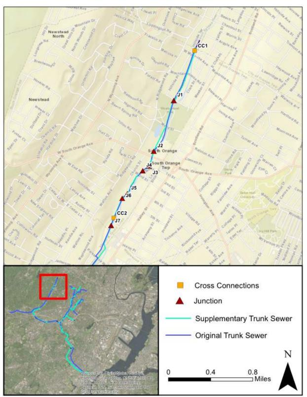
Figure 2-8 Locations of Cross Connections and Junctions between Original and Supplementary Trunk Sewers – Northwest Portion of Service Area
