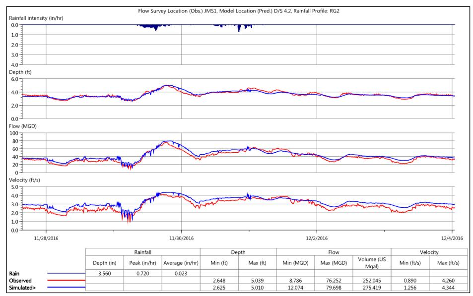
Figure 4-13 Calibration Time Series Plots at Meter JMS1 for the 11/29-30/16 Calibration Event
