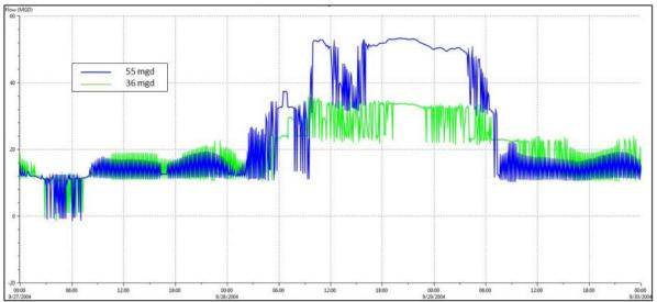
Figure 7-24 Comparison of Simulated TAPS Discharge at Higher Pumping Rate
