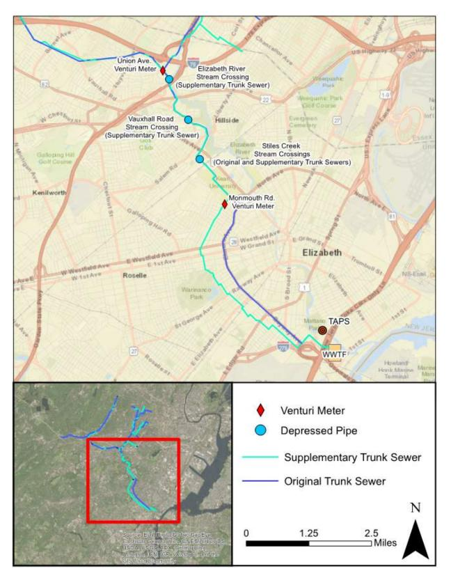
Figure 2-12 Locations of Venturi Meters and Depressed Pipes within the JMEUC Trunk Sewer System
