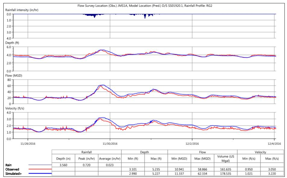
Figure 4-14 Calibration Time Series Plots at Meter JMS1A for the 11/29-30/16 Calibration Event
