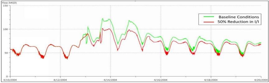
Figure 7-22 Comparison of Simulated WWTF (Primary Effluent) Flow Rate with 50% System Wide RDII Reduction (April 2004)
