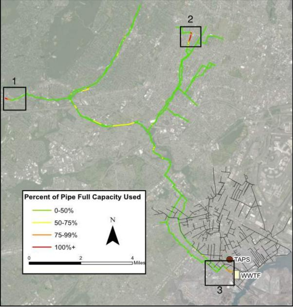
Figure 7-2 JMEUC Trunk Sewer Capacity During Dry Weather
