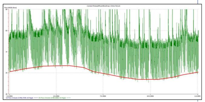
Figure 7-1 Seasonal Trend in Base Groundwater Infiltration at WWTF (Primary Effluent)
