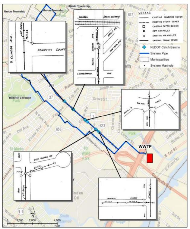
Figure 2-3 NJDOT Catch Basin Connections to the JMEUC Original Trunk Sewer
