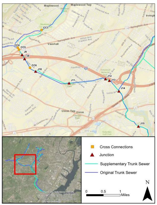
Figure 2-9 Locations of Cross Connections and Junctions between Original and Supplementary Trunk Sewers – North-Central Portion of Service Area
