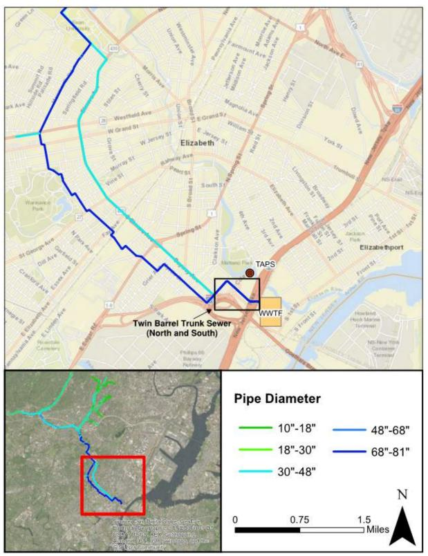
Figure 2-7 JMEUC Trunk Sewer Pipe Sizes and Shapes – Southeast Portion of Service Area
