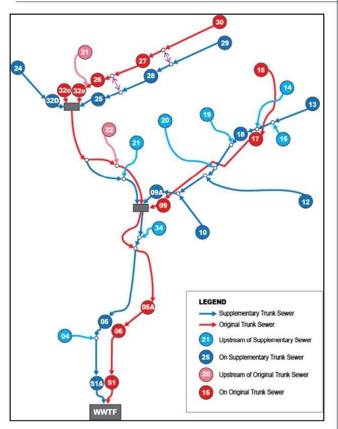
Figure 4-5 JMEUC Flow Meter Connectivity
