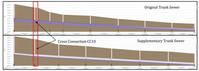
Figure 7-3 Peak HGL of Surcharged Segments #2 during Dry Weather – Trunk Sewers
