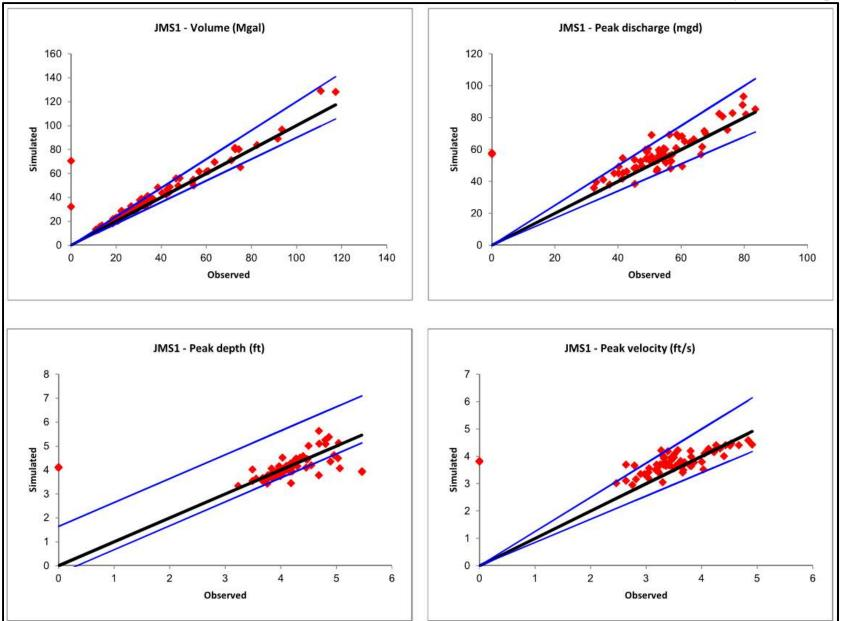
Figure 4-15 Scatter Plots Showing a Comparison of Observed and Simulated Data at Meter JMS1 for the 72 Rainfall Events Identified during the Calibration Period
