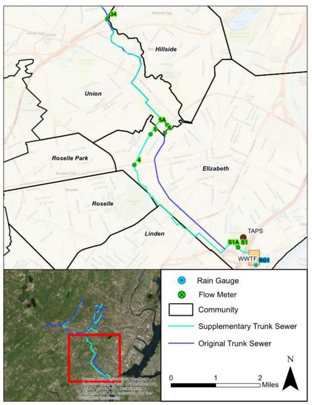
Figure 4-4 Flow Meter and Rain Gauge Locations – Central and Southeast Service Area
