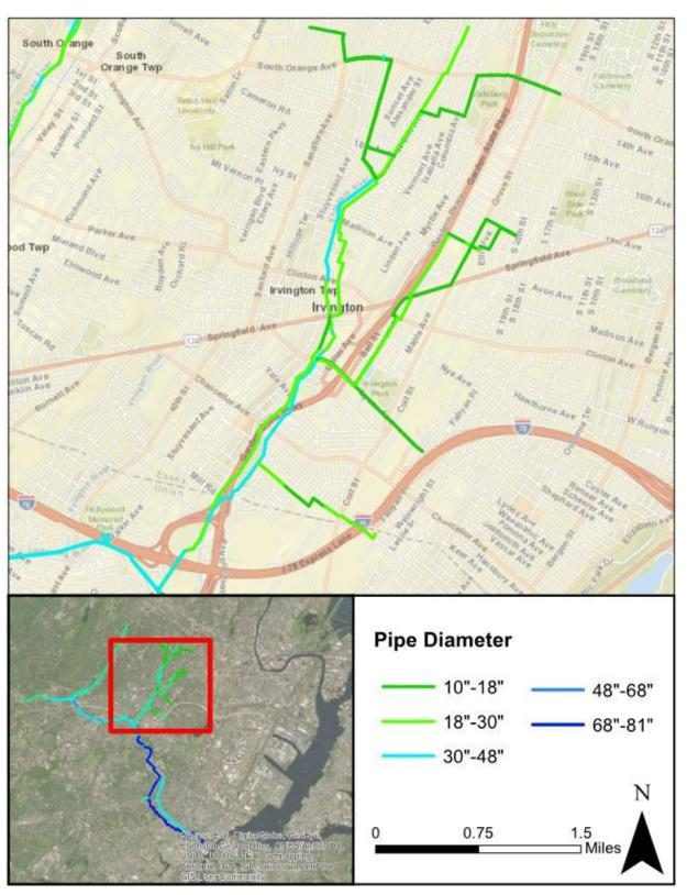
Figure 2-5 JMEUC Trunk Sewer Pipe Sizes and Shapes – Northern Portion of Service Area
