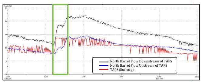
Figure 7-20 Peak flow timing for the Elizabeth combined sewer system and for the upstream sanitary sewer portions of the JMEUC trunk sewer system
