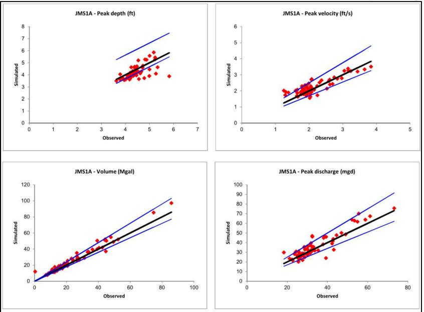
Figure 4-16 Scatter Plots Showing a Comparison of Observed and Simulated Data at Meter JMS1A for the 72 Rainfall Events Identified during the Calibration Period
