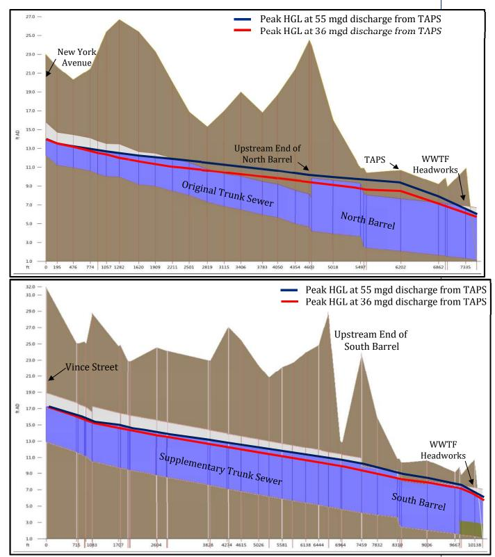
Figure 7-26 Comparison of Peak HGL along the Trunk Sewers (September 28, 2004 Storm)
