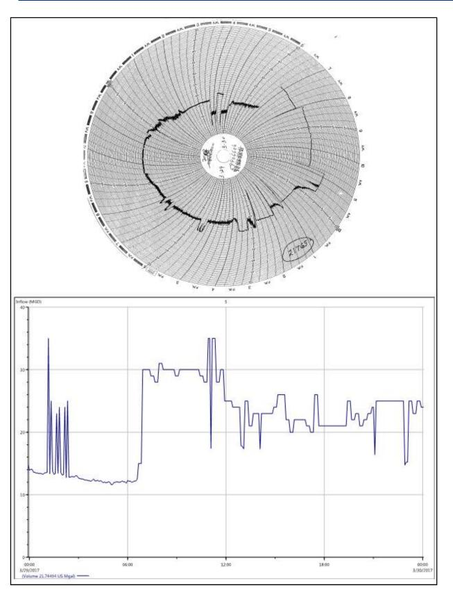
Figure 4-6 Example of Circular Chart Data and Digitized Time Series for 3/29/17 – 3/30/17
