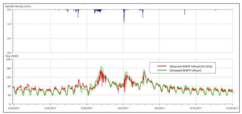
Figure 7-7 Primary Effluent at JMEUC's the WWTF during March and April 2017
