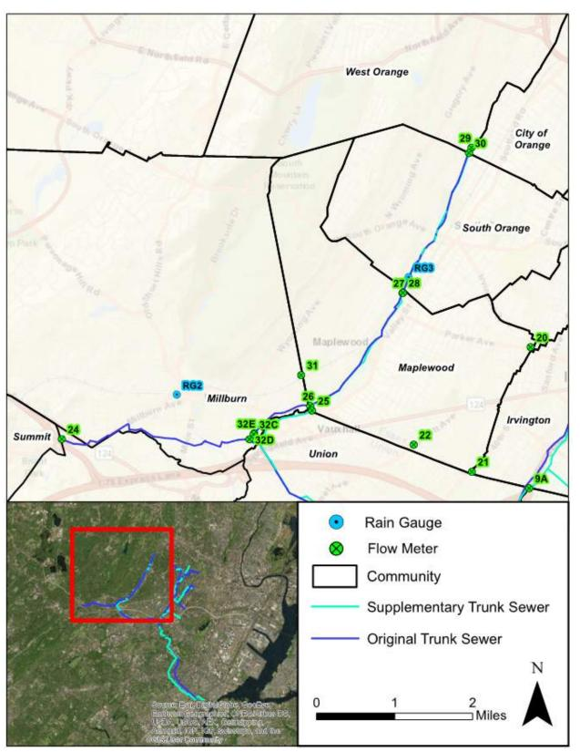
Figure 4-2 Flow Meter and Rain Gauge Locations – Northwest Service Area
