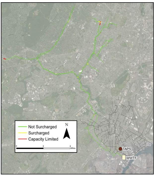
Figure 7-21 Maximum Surcharge State in 2004 Typical Year with System Wide 50% RDII Reduction
