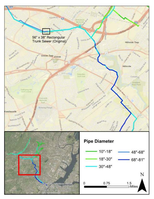
Figure 2-6 JMEUC Trunk Sewer Pipe Sizes and Shapes – Central Portion of Service Area
