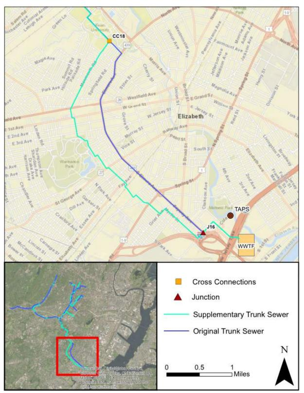
Figure 2-11 Locations of Cross Connections and Junctions between Original and Supplementary Trunk Sewers – Southeast Portion of Service Area
