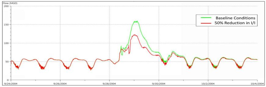
Figure 7-23 Comparison of Simulated WWTF (Primary Effluent) Flow Rate with 50% System Wide RDII Reduction (September 2004)
