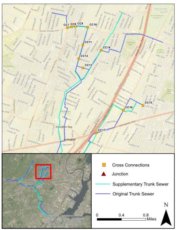
Figure 2-10 Locations of Cross Connections and Junctions between Original and Supplementary Trunk Sewers – Northern Portion of Service Area
