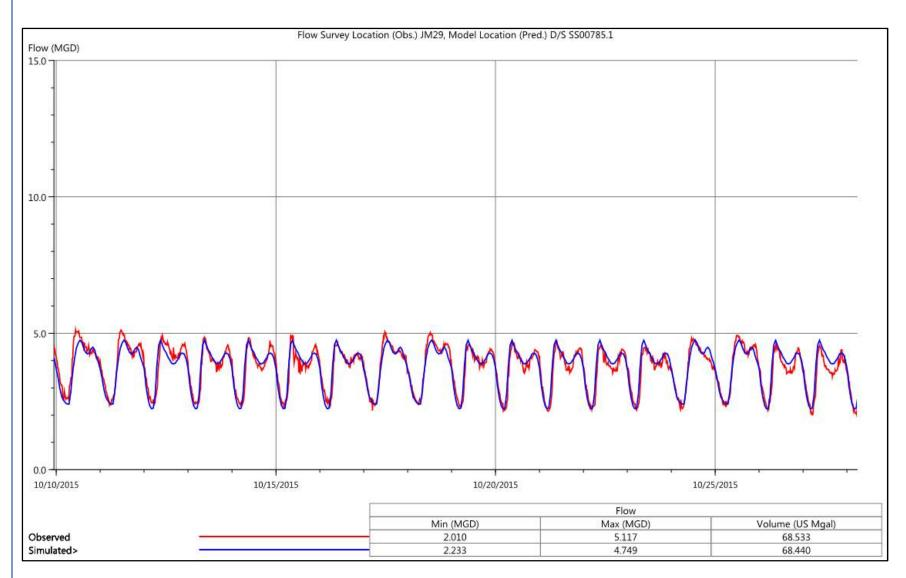
Figure 4-8 Calibrated DWF at Meter JM29 During Extended Dry Period in October 2015
