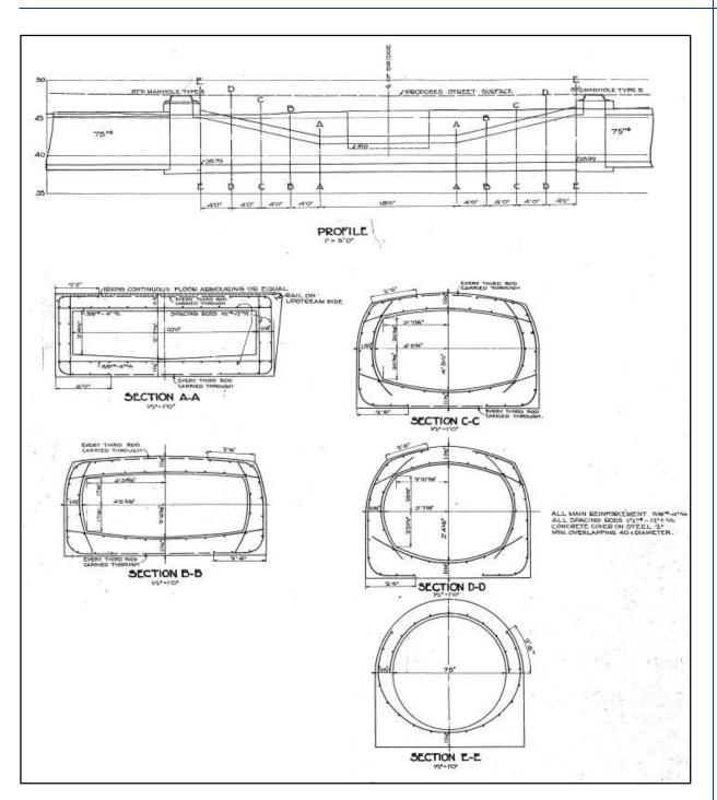
Figure 2-14 Profile and Cross-Sectional Views of the Depressed Pipe Located at Vauxhall Road
