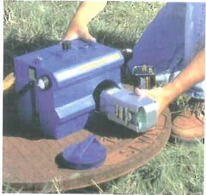
Two alkaline lantern batteries provide power for up to 15 months.
