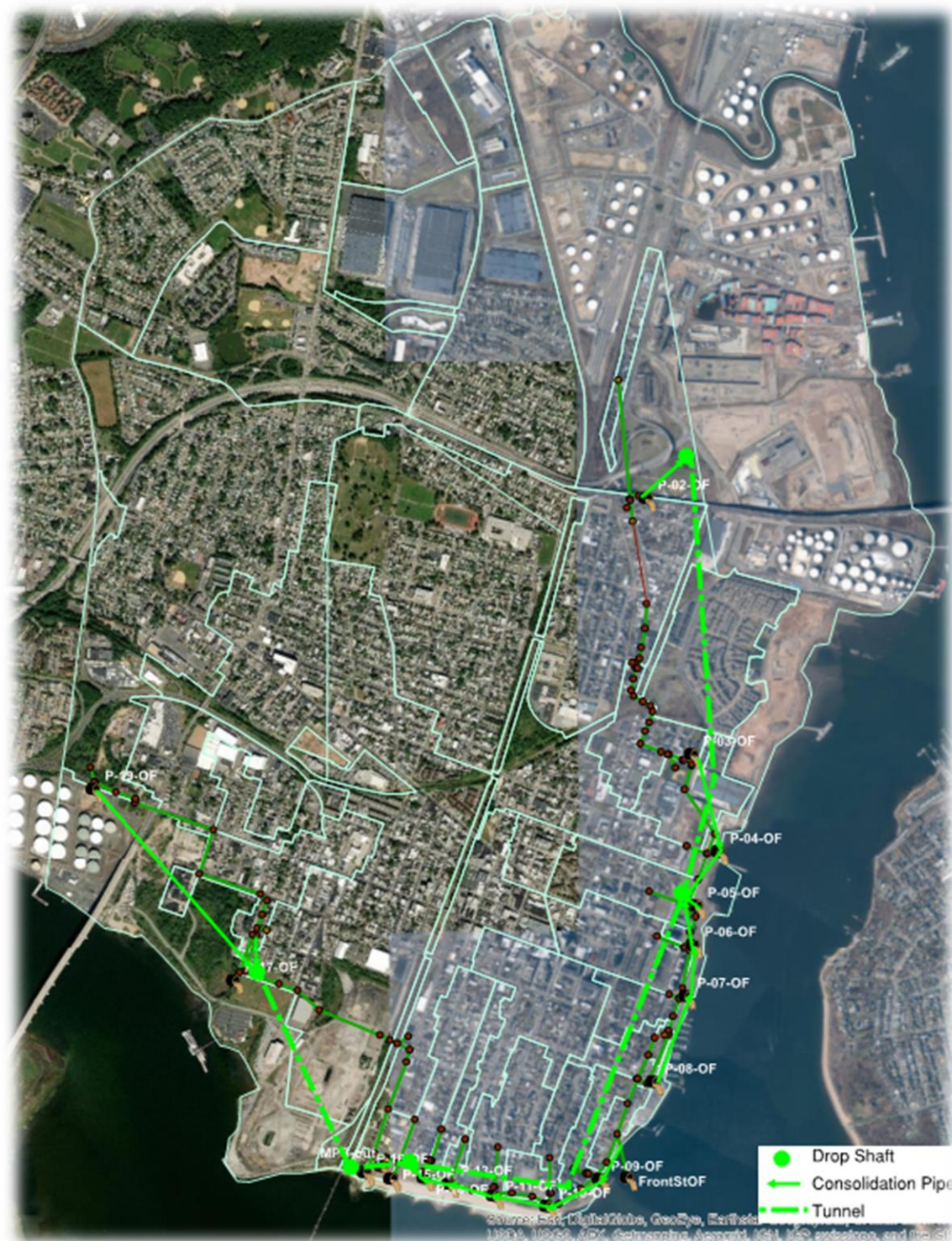
Figure 5-5 - Conceptual Layout for Deep Tunnel Storage
