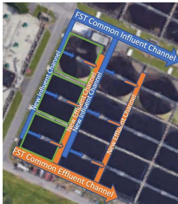
Figure 4-24. Alternative FC flow path
