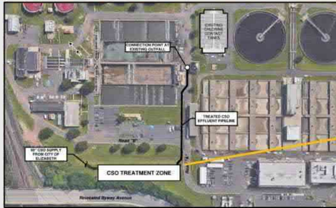
General Site Layout for New CSO Treatment Train at JMEUC WWTF
