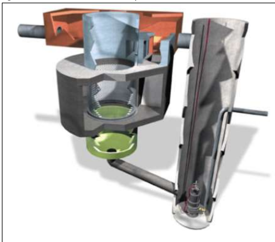
Figure 2-11 - Cross Section of a SanSep Unit
