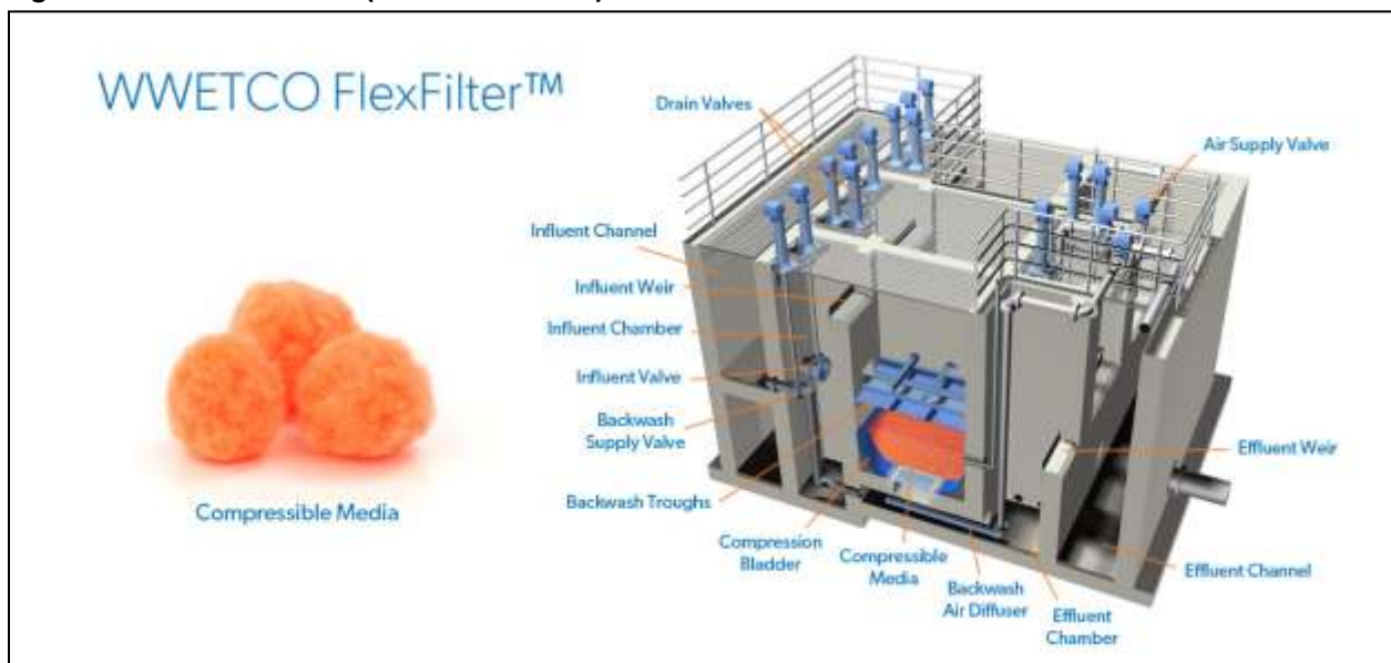
Figure 2-20 - FlexFilter Unit (Source: WesTech)
