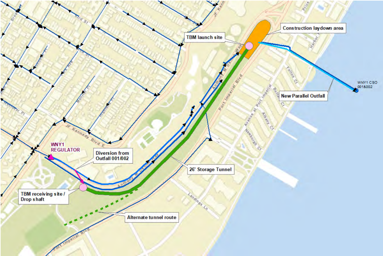
Figure 4-6. Conceptual Tunnel Layout – Construction Stage
