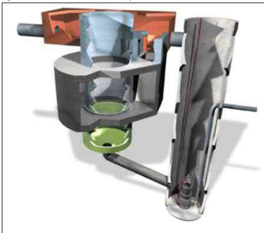
Figure 2-11 - Cross Section of a SanSep Unit
