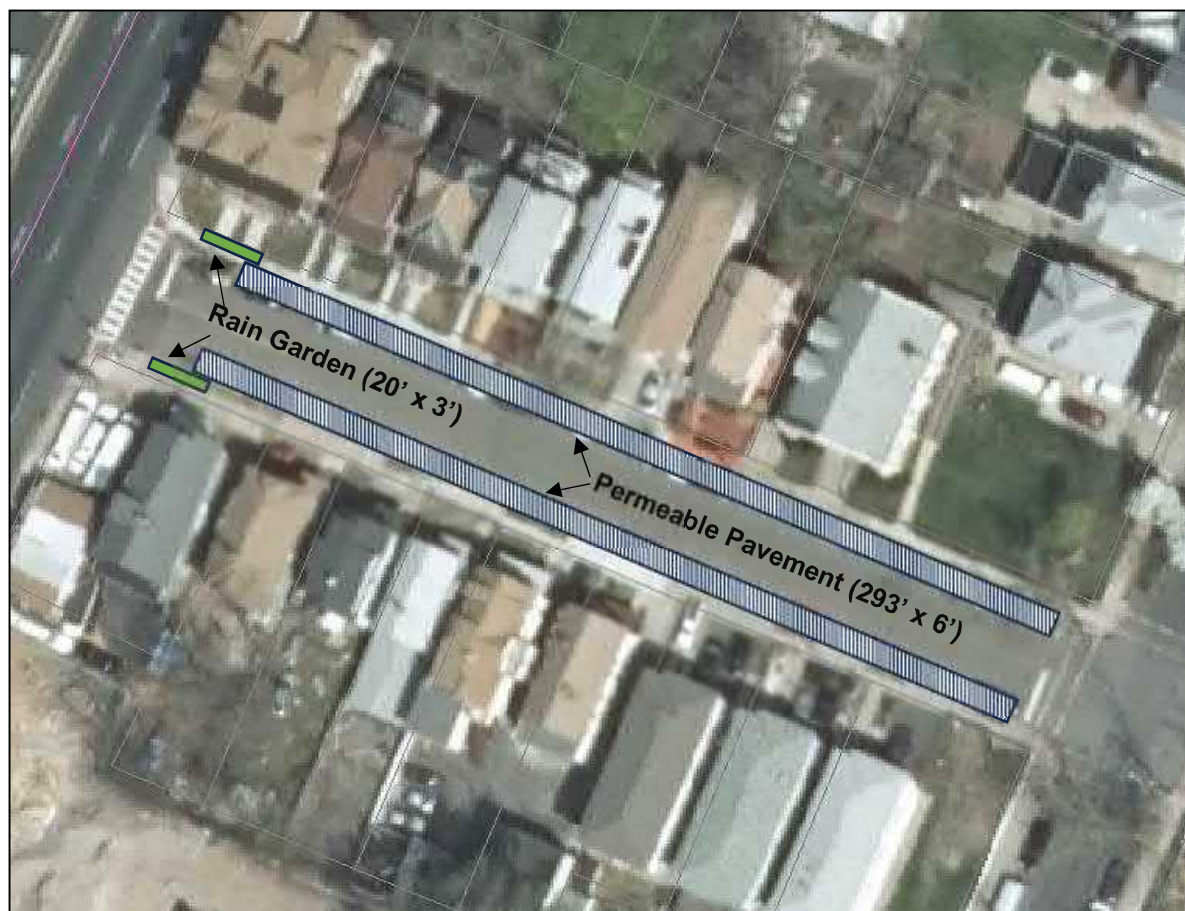
Figure 7-32: Typical street segment with green stormwater infrastructure
