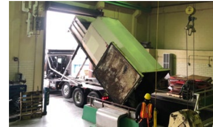
1. Compactor Dumping Food Waste
