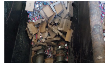
3. Receiving Hopper Processing Cans
