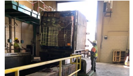
2. Walking Floor Dumping Material
