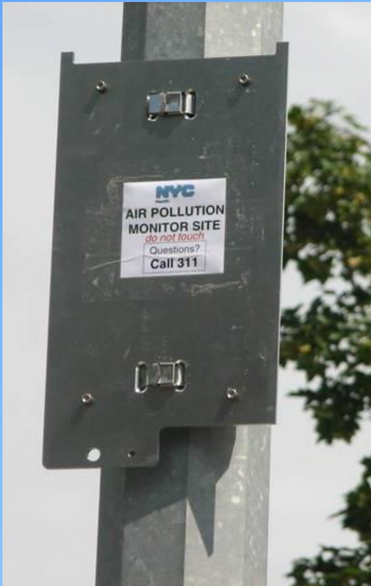
Pre-installed mounting plate for rapid deployment and retrieval
