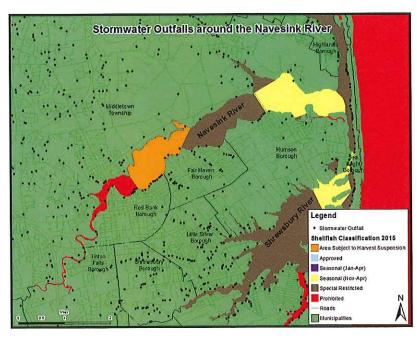
municipal infrastructure. Storm drains along roads collect the runoff and transmit it to stormwater outfalls. The outfalls discharge the runoff into streams, bays, oceans, and other bodies of water. They are often found in urban areas, and are especially common within lagoon communities. The first flush after a rain event often carries the most pollutants.
