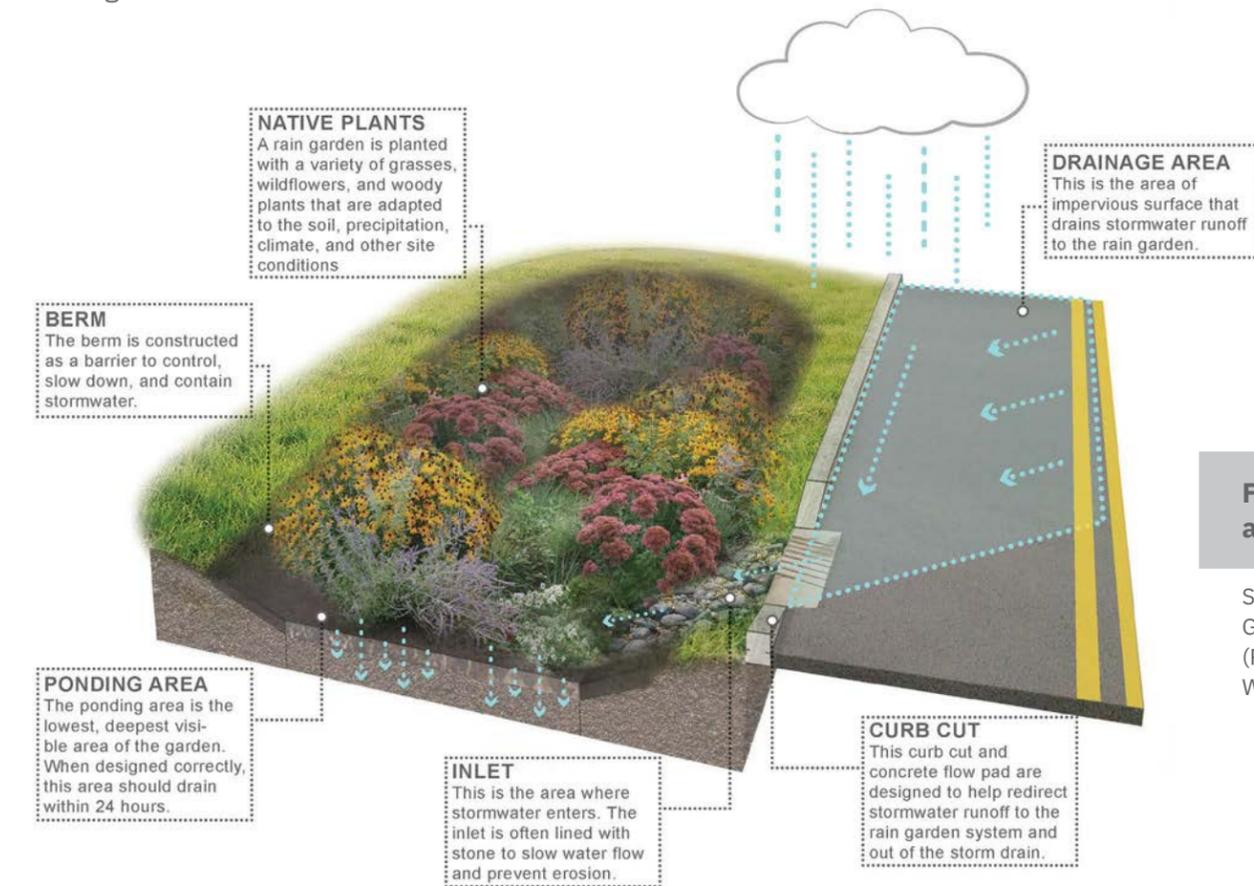
**Figure 6.7 Rain Garden and Bioretention Diagram**
