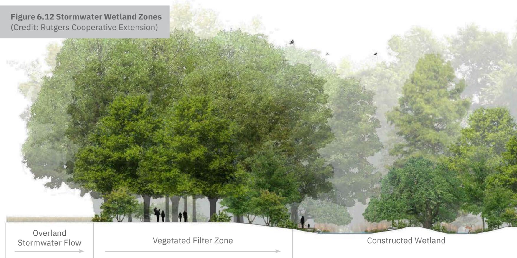
Stormwater wetlands support a variety of plants and aquatic life. The design of these systems needs provide a range of hydrologic zones that capture and filter stormwater runoff through settling, plant uptake, and other biological processes. Critical considerations when planning or proposing a stormwater include:
