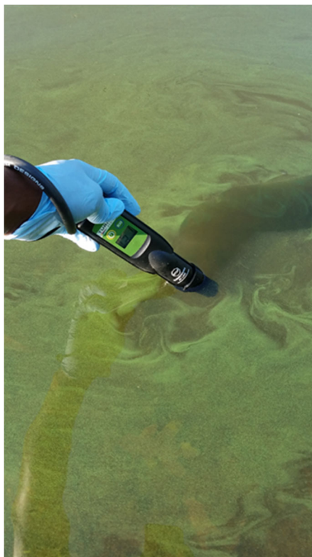
Figure 4. Field Fluorometer For Measuring Phycocyanin
