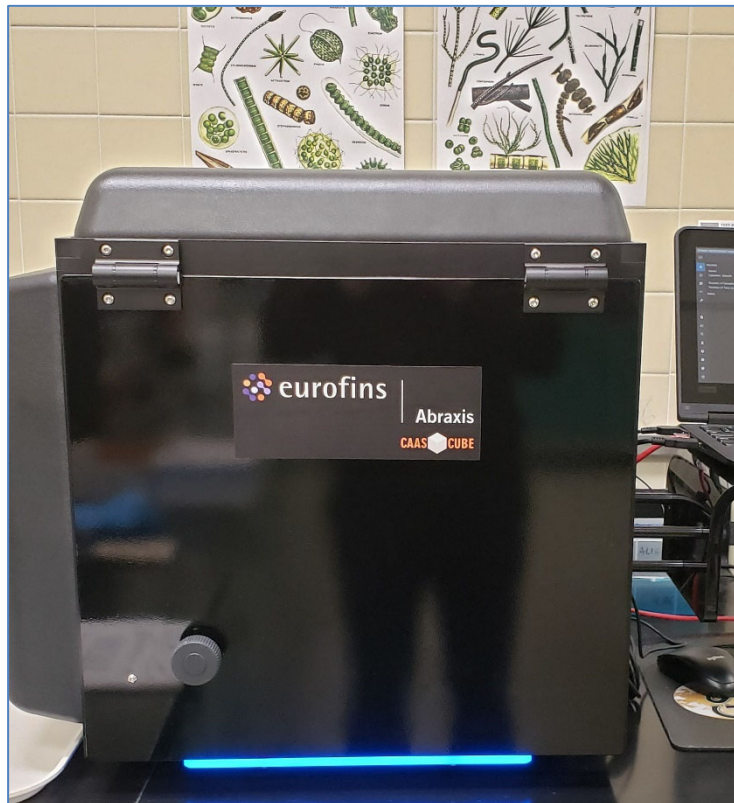
Figure 7. Cyanotoxin Automated Analyzer System (CAAS)
