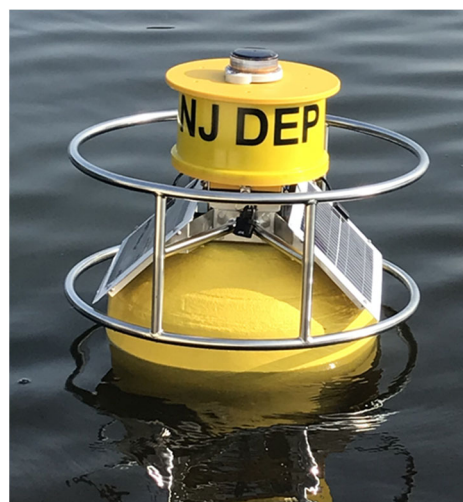
Figure 5. Continuous multi-parameter meter.
