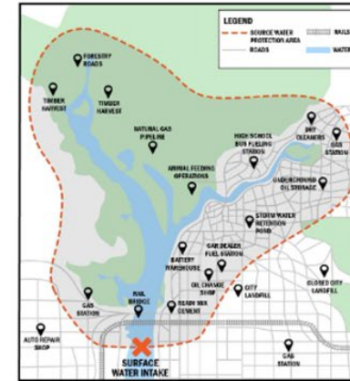
Inventory Potential Sources of Contamination
